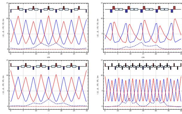
Figure 2: Lattices with two-fold symmetry and 22 cells (lower right) and four-fold symmetry with 20 cells. Only one superperiod (out of two respectively four) is shown.
