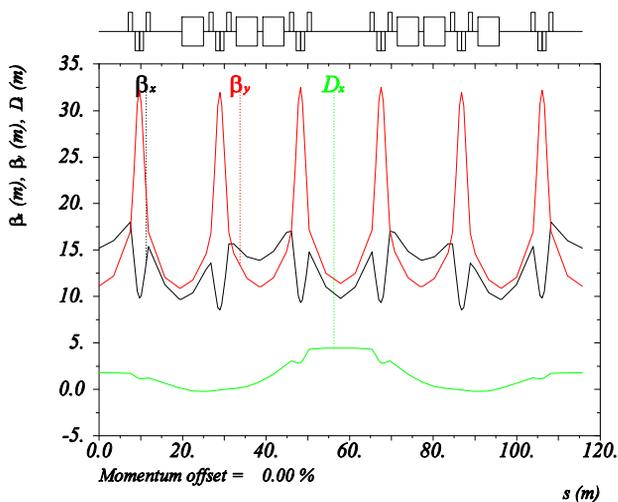
Figure 1: Betatron functions for one superperiod of the 3.2-9.6 GeV RCS booster for the Neutrino Factory.
