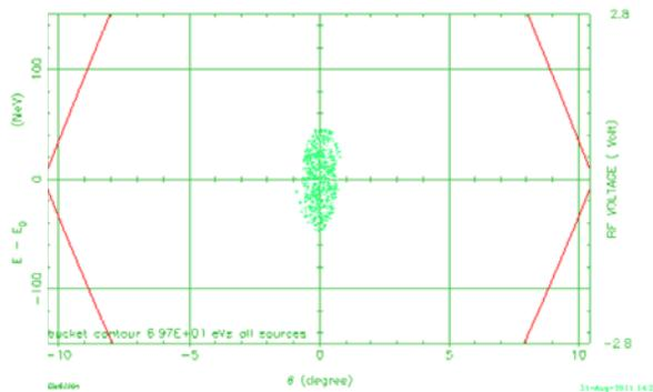
Figure 3: Showing the initial, mid-point and concluding longitudinal phase-space diagrams. The scale in degrees is divided by the harmonic number.
