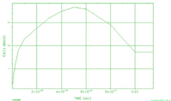
Figure 2: Voltage as a function of time in the dedicated 3.2-9.6 GeV RCS booster for the NF.
