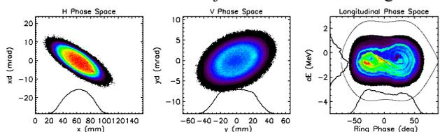
Figure 2: Beam distributions in  $(x, x')$ ,  $(y, y')$ ,  $(\phi, \Delta E)$ , at the end of injection.
