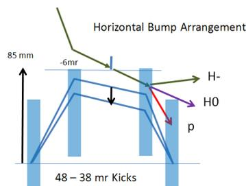
Figure 1: Schematic of 180 MeV injection straight.
