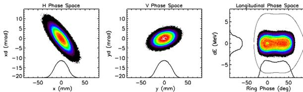
Figure 3: Beam distributions  $(x, x')$ ,  $(y, y')$ ,  $(\phi, \Delta E)$ , 7.3 ms through the 10 ms acceleration process.
