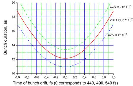
Figure 1: Dependence of bunch duration on time in the laboratory system;  $\lambda = 10 \mu\text{m}$ ,  $E_{qst} = 1 \cdot 10^9 \text{ V/cm}$ ,  $E_{L0} = 1.6 \cdot 10^9$ ,  $v_{\parallel} = 1.64 \cdot 10^{10} \text{ cm/s}$ ,  $I_0 = 13 \text{ mA}$ ,  $I_{max} = 10 \text{ A}$ , number of electrons with bunch  $N_e = 760$ ,  $d_{drift} = 80 \mu\text{m}$ .
