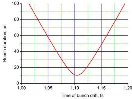
Figure 2: bunch duration on time in the laboratory system;  $\lambda = 1 \mu\text{m}$ ,  $v_0 = 2,5 \cdot 10^9 \text{ cm/s}$ ,  $v_{\parallel} = 3 \cdot 10^9 \text{ cm/s}$ ,  $I_0 = 10 \text{ mA}$ ,  $I_{max} = 1.5 \text{ A}$ , number of electrons with bunch  $N_e = 90$ .
