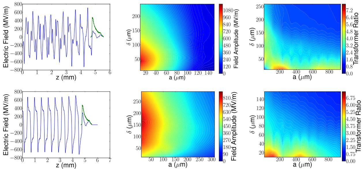
Figure 2: Wakefield (blue trace) produced by a 500-pC bunch with ramped current distribution (green trace) [left column], scan of the peak accelerating field ( $E_+$ ) [middle column], and scan of the transformer ratio ( $\mathcal{R}$ ) [right column], in the  $(a, \delta)$  parameter spaces. The top and bottom rows respectively correspond to cylindrical and slab DLWs. The wakefield plotted in the left column correspond to  $(a, \delta) = (20, 60) \mu\text{m}$ .
