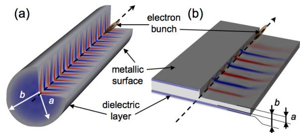
Figure 1: Geometries of interest: (a) An electron bunch passes through a cylinder with inner radius  $a$ , and outer radius  $b$ . (b) Similarly an electron bunch passes through a slab-symmetric geometry of inner length  $a$ , and outer length  $b$ . In both instances, the dielectric material is located in the region  $\delta = b - a$ , the geometries are surrounded by a conducting sheet, and the region  $< a$  is vacuum.
