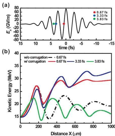
Figure 3: (a) Relative delays between the laser pulse and the electron test particles launched in the simulation. (b) Dependence of the electron test particle kinetic energy on the propagation distance for particles launched from the origin at different delays relative to the laser pulse.
