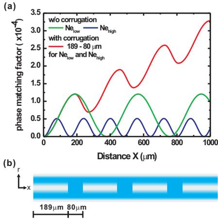
Figure 1: (a) Dependence of phase matching factor  $f$  on propagation distance for uncorrugated waveguides with  $N_{e,high} = 1.25 \times 10^{19} \text{ cm}^{-3}$  and  $N_{e,low} = 2.25 \times 10^{18} \text{ cm}^{-3}$  and corrugated waveguide with periodic  $N_{e,low}$  and  $N_{e,high}$  modulation. (b) Plots for the structure of the corrugated waveguide for QPM calculation and PIC simulation.
