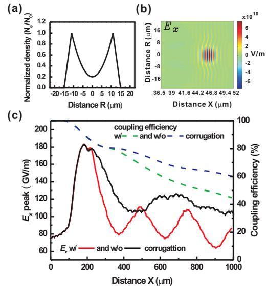
Figure 2: (a) Electron density profile normalized to  $N_{e0} = 1.25 \times 10^{19} \text{ cm}^{-3}$  for the plasma waveguide in the PIC simulations. (b) Snapshots for the longitudinal electric field  $E_x$  at the focal position. (c) Dependence of the longitudinal electric field  $E_x$  peak value and laser pulse energy coupled efficiency in the plasma channel on the propagation distance in cases with and without corrugation.
