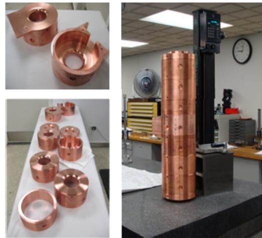
Figure 2: Machined copper cells for new linac tank, and cell stacking prior to brazing.
