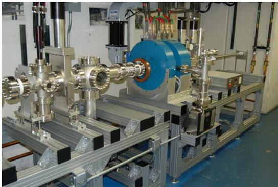
Figure 1: The new AWA RF gun (between the blue solenoids) commissioned, initially with a copper photocathode, which was later replaced with a Cesium Telluride photocathode.
