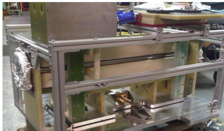
Figure 3: Kicker magnet ready for installation in the BSY.
