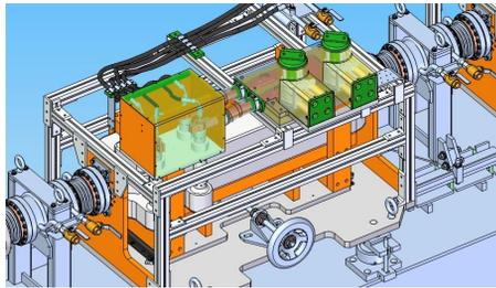
Figure 2: (top) Layout of the 4 kicker magnet system to kick the beam into ESA; (bottom) magnet assembly.
