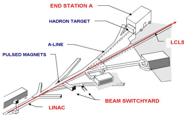
Figure 1: SLAC complex at the end of the 2-mile long linac. Pulsed magnets are used to kick the beam into ESA.
