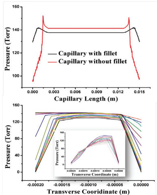
Figure 3: Comparison of pressures along the longitudinal direction (top) and radial pressures near the end of capillary (bottom) for capillary with and without fillet.
