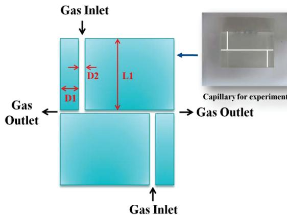
Figure 1: A gas-filled capillary waveguide for simulation.
