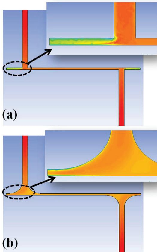
Figure 2: Turbulence level of capillaries with and without fillet.
