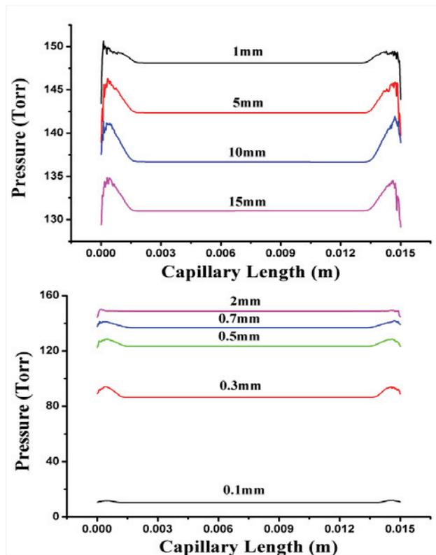
Figure 4: Pressures under various inlet lengths (top) and inlet widths (bottom).
