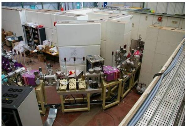
Figure 2: View of ECR deuteron source and its associated LEBT lines mounted at CEA/Saclay.
