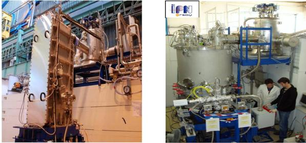
Figure 4: The SPIRAL2 superconducting cryomodules (left:  $\beta_0=0.07$ - 1cav, right:  $\beta_0=0.12$ - 2cav).
