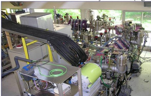
Figure 3: View of PHOENIX-V2 source and its associated LEBT1 line mounted at IN2P3-LPSC/Grenoble
