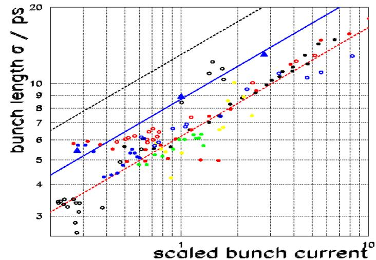
Figure 2: Scaled bursting threshold current  $\tilde{I}$  and bunch length  $\sigma_0$ . Blue line: theory; blue triangles: BESSY II data; circles: MLS data. All data are measured with a liquid He cooled InSb detector of one MHz frequency response.
