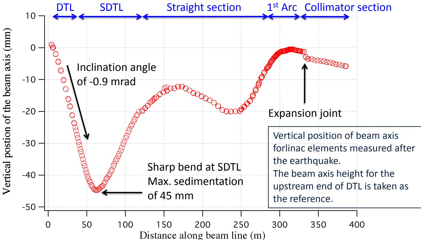
Significant deformation of the linac tunnel necessitated us to conduct urgent realignment.
