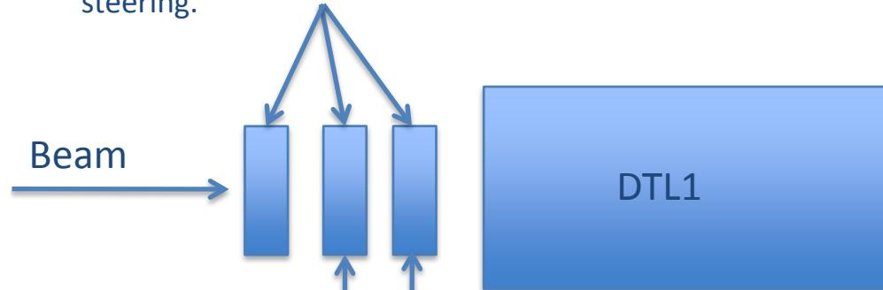
The strengths of the last two steerings have been adjusted to maximize the transmission efficiency for the entire DTL.
