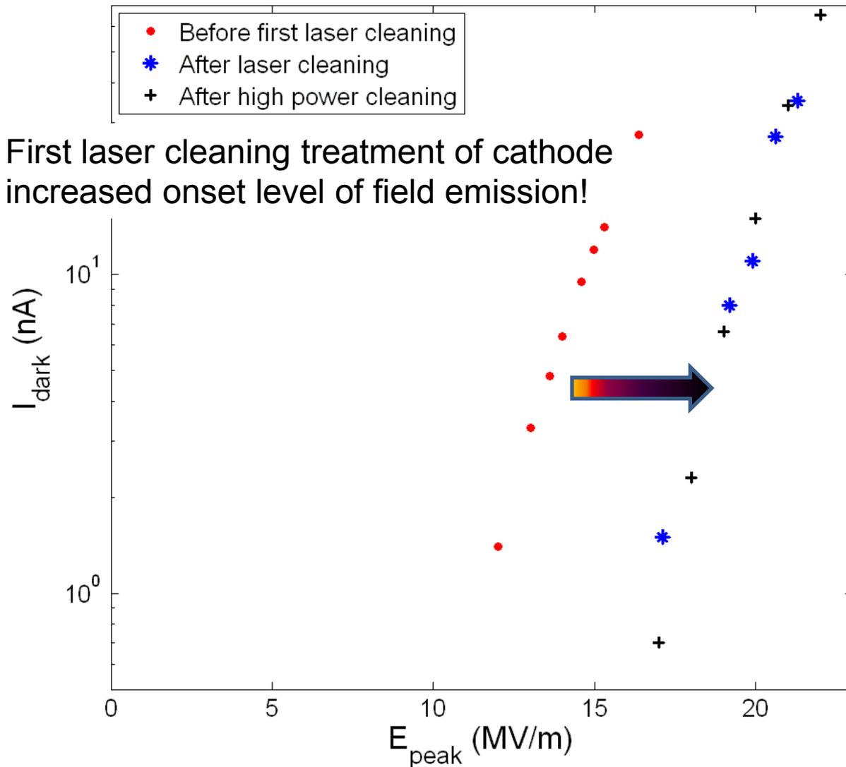
First laser cleaning treatment of cathode increased onset level of field emission!
