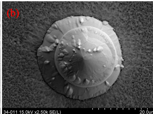
SEM images of comparable samples show droplets and tip on tip like structures
