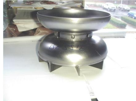
Large grain cavity backwall for cathode
