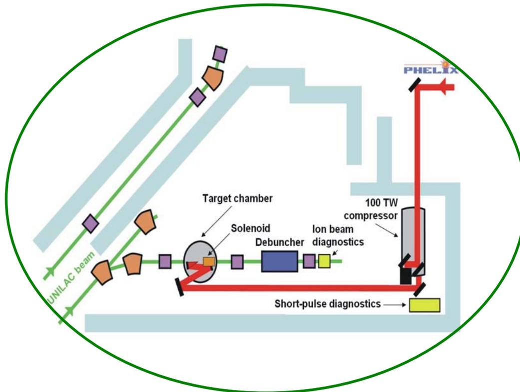
The LIGHT test stand integrated to the UNILAC experimental beam line.
