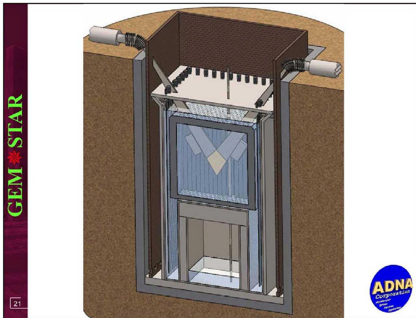
Conceptual design of the GEM\*STAR reactor in its underground placement. The vertical dimension is about 30 ft. The gray box is the graphite reflector for the core. Horizontal beams from two accelerators are shown at the top being bent by magnets about 45 degrees into the core where both strike a uranium metal target shown schematically in the center of the core.
