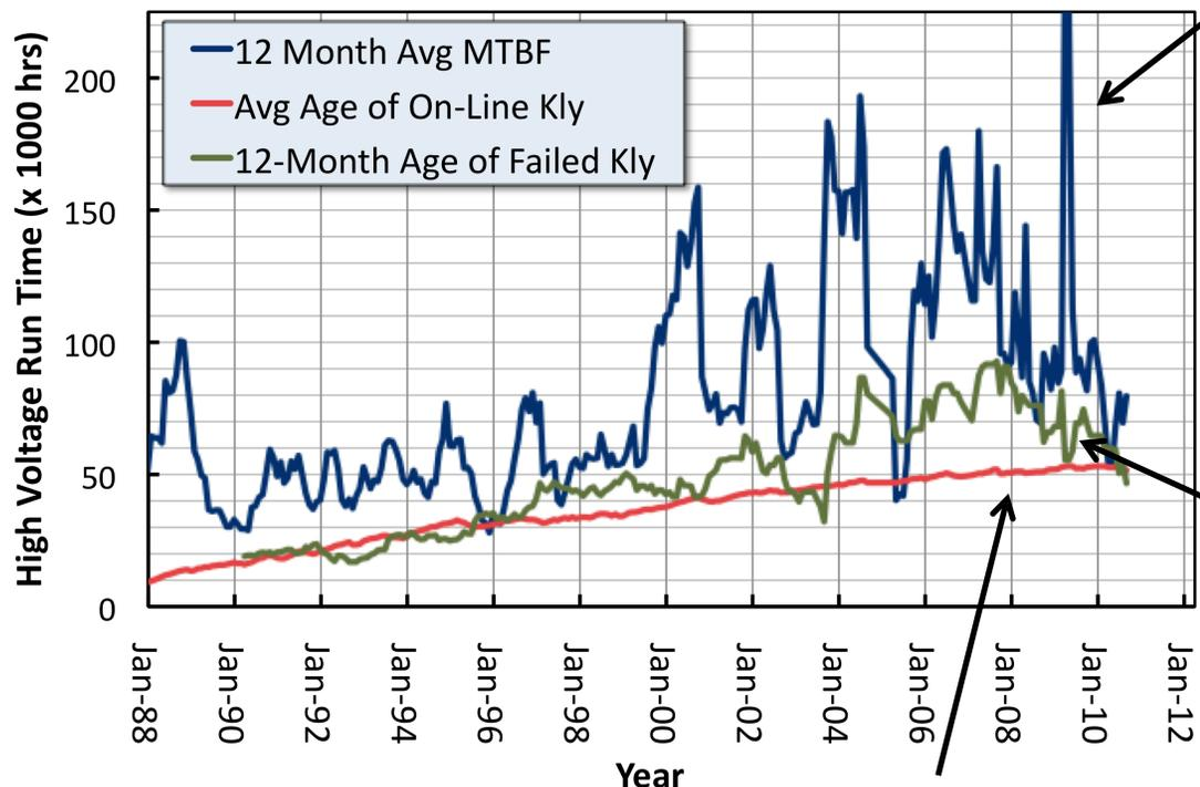
**12 Month Avg MTBF:** total HV hours accumulated on all klystrons during the previous 12 months divided by the total number of failed klystrons during the same period – **80-90,000 hr**
