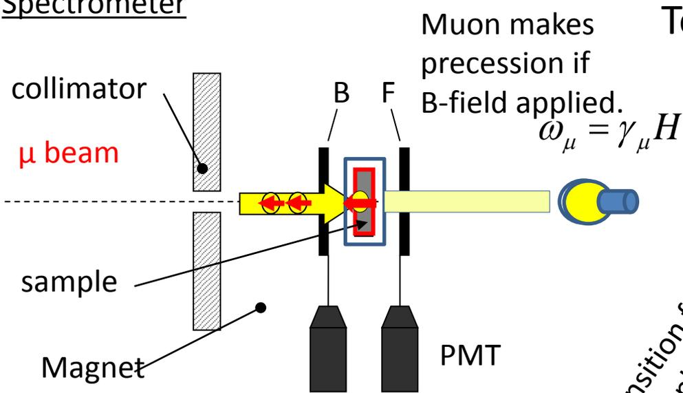
As the direction of decayed positron depends on muon spin, forward/backward asymmetry of PMT indicates muon spin in target material
