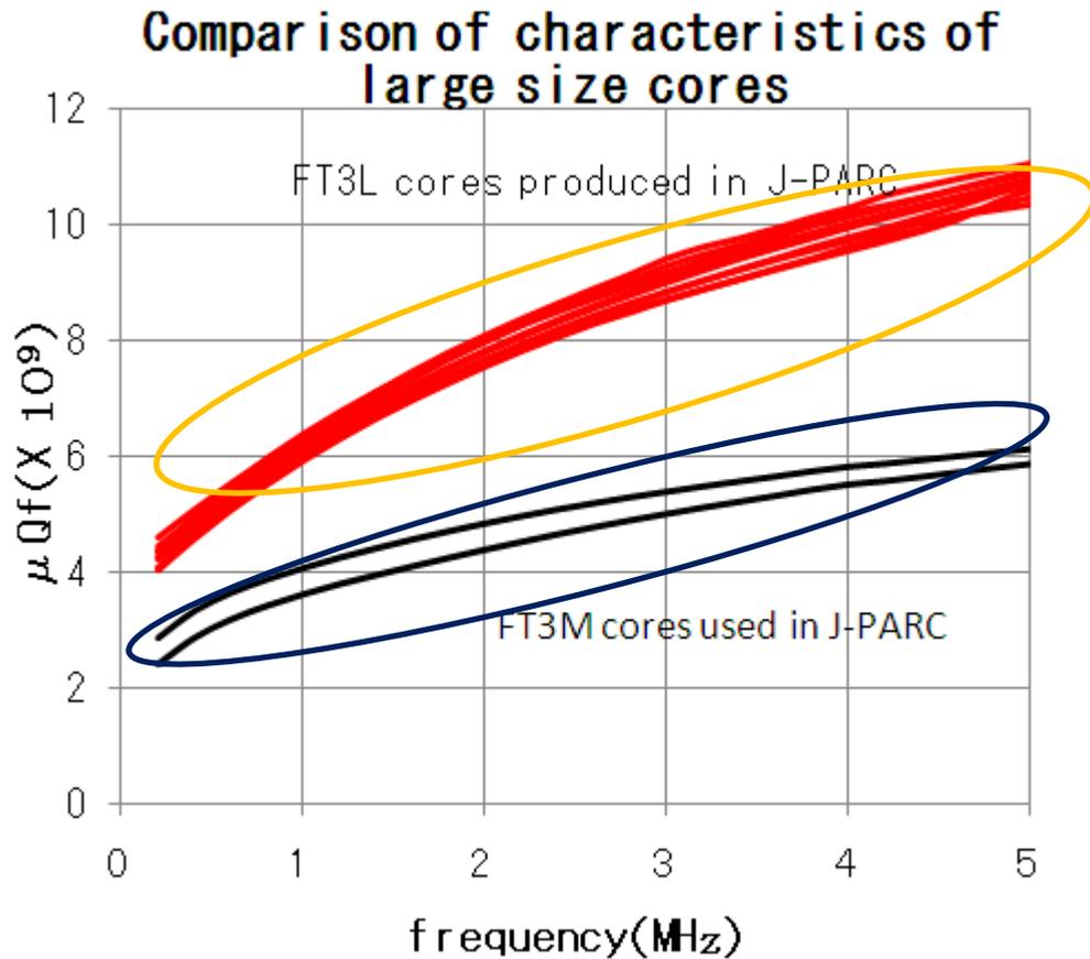
$\mu Qf$  is given by core impedance divided by a core form factor.
