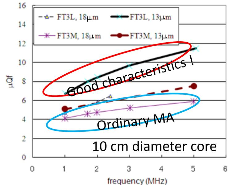
If easy-magnetized axis of crystalline is parallel to RF flux, it is bad for RF use.
