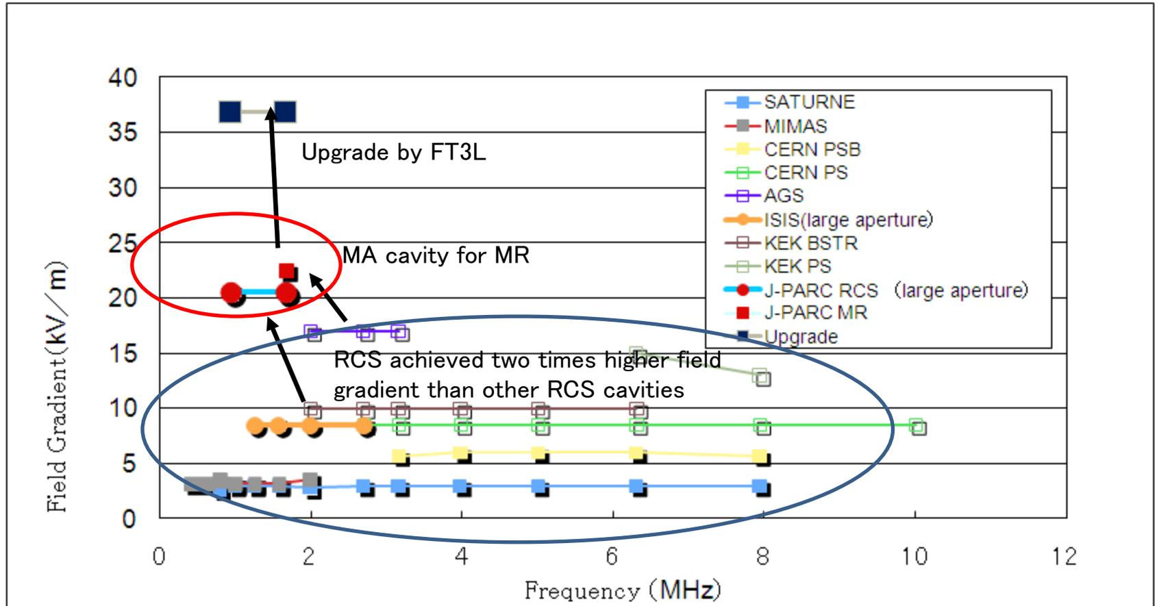
**Development of FT3L large-size cores for accelerators will help to develop and improve other proton/ion rings.**
