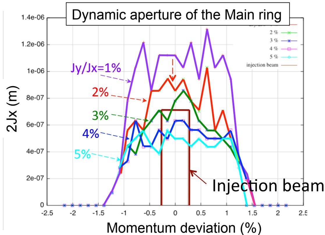
If  $J_y/J_x < 2\%$ , the beam is safely injected in the Main ring.
