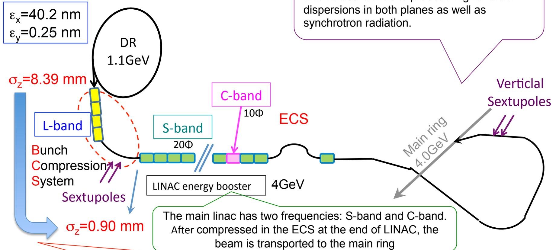
The bunch length is one-order reduced by the BCS to match the S-band frequency of the linac. We should use an L-band accelerating structure for longitudinal focusing such a long bunch.
