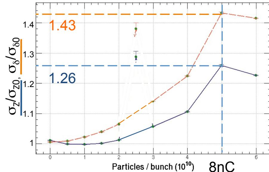
Anyway these enlargements of bunch length and energy spread are within acceptable range for the injection.
