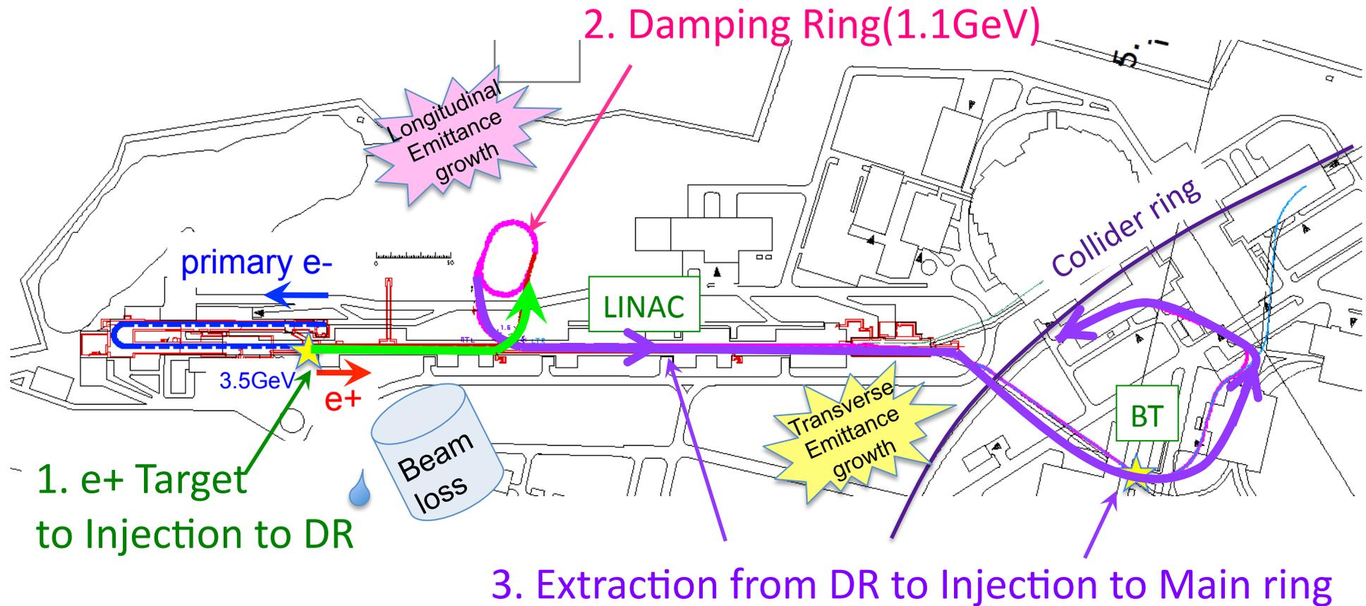
We did **the overall tracking simulation** from the  $e^+$  generation to Main ring injection, assuming **8nC** charge.
