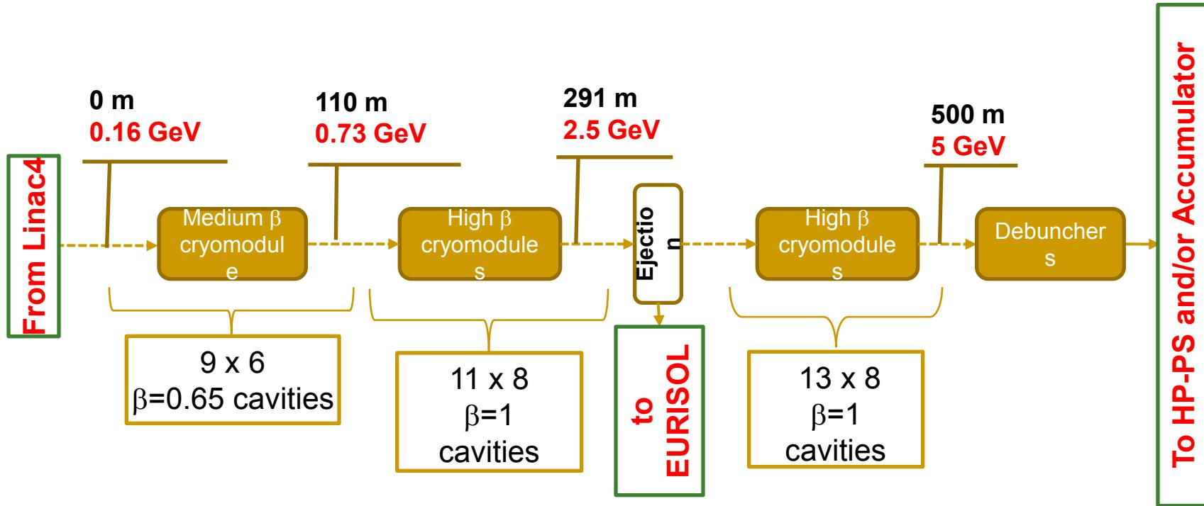
Segmented cryogenics / separate cryo-line / room temperature quadrupoles:
