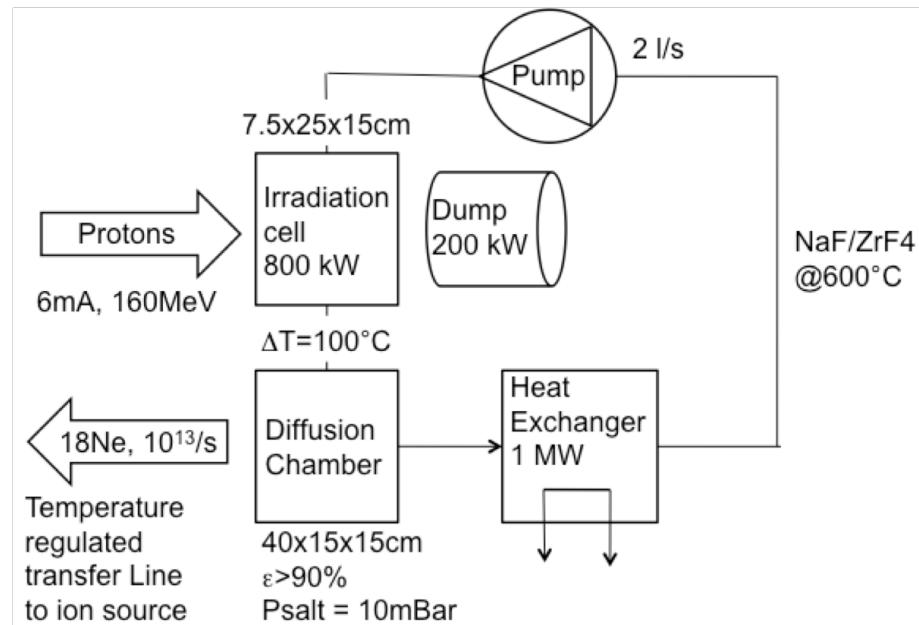
$^{18}\text{Ne}$  production rate estimated to  $1 \times 10^{13}$  ions/s (dc) for 960 kW on target.
