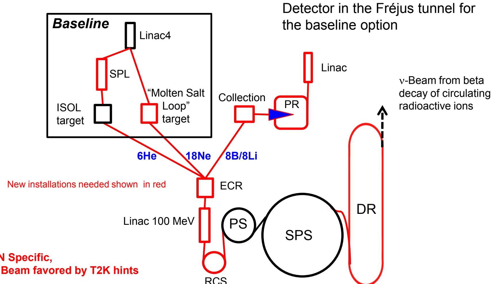
Decay Ring:  $B\beta \sim 500 \text{ Tm}$ ,  $B = \sim 6 \text{ T}$ ,  $C = \sim 6900 \text{ m}$ ,  $L_{ss} = \sim 2500 \text{ m}$ ,  $\gamma = 100$ , all ions
