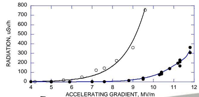
He processing by ASTeC RF + cryogenic groups with assistance from T. Powers (Jlab)
