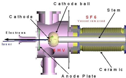
Ceramic insulator electrically insulates HV cathode ball and stem.
