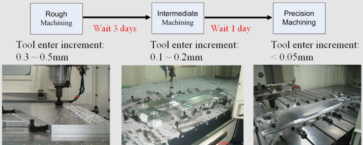
CNC Machining Processes (sprayed with pure alcohol)
