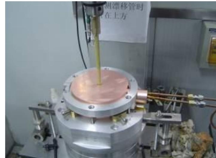
Sakae coil and quadrupole at rotating coil measurement
