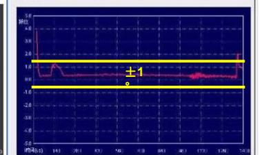
FPGA based digital LLRF control system with effective control of ph & ampl.
