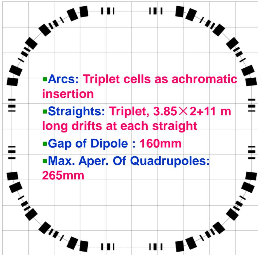
Lattice consists of 16 triplet cells, with a gap in the middle of arc and dispersion free straight section .
