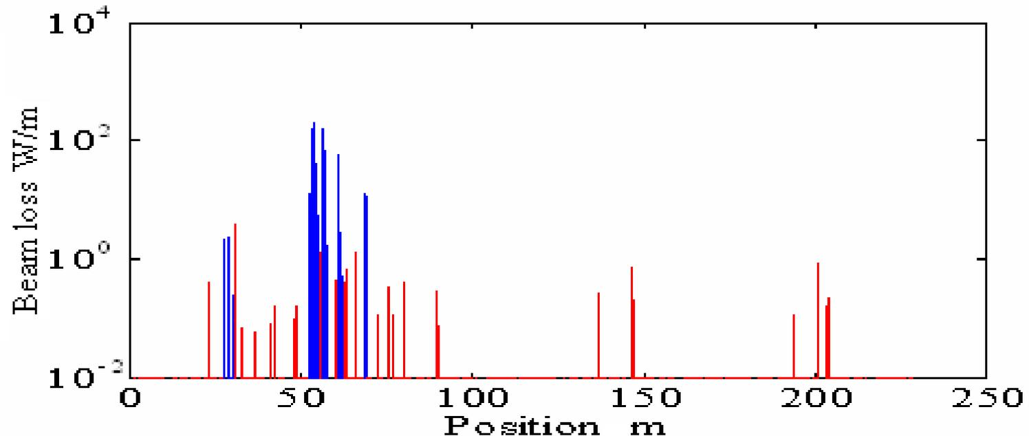
**Beam loss distribution in the RCS with transverse and momentum beam collimation, total beam loss is about 5%, and the collimation efficiency is more than 96%**
