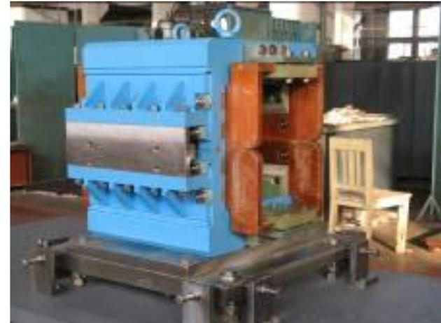
A pulsed power supply with 18kA output current in maximum during injection time of  $500\mu\text{s}$  connected with the bump magnet for the magnet measurement.
