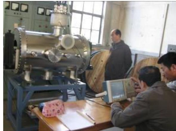
The pulse power supply uses Blumlein type pulse forming network to get a short pulse with a current of 5840A and a flat top of better than  $\pm 1.5\%$
