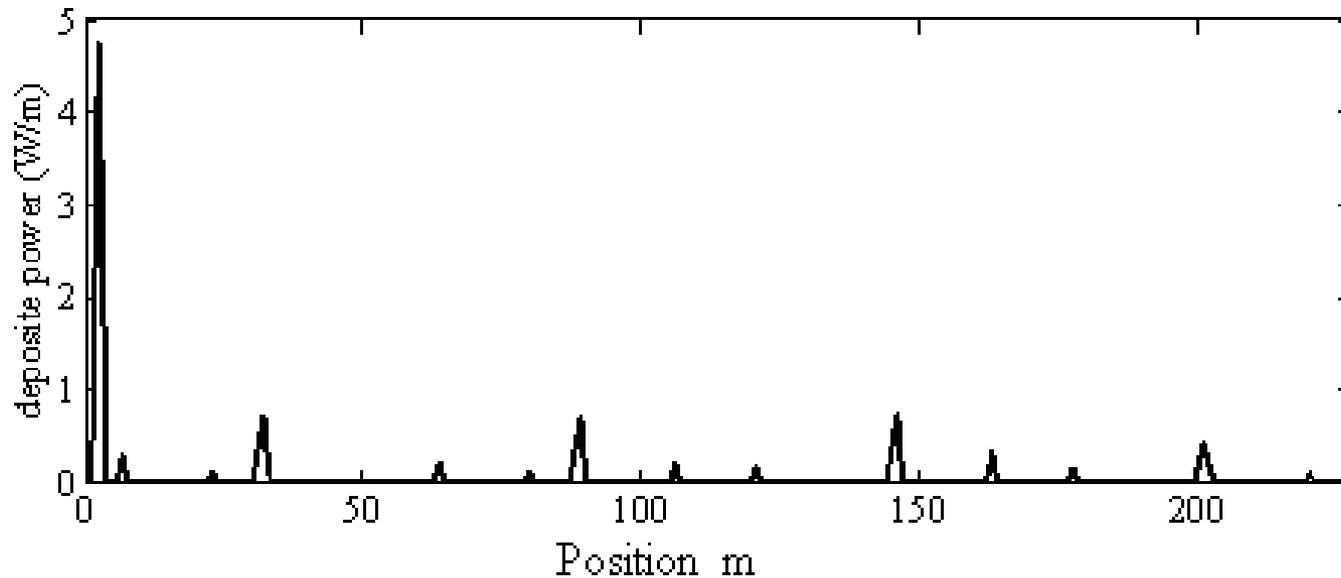
**In case of no beam collimation, the total beam loss is small, but the maximum local beam loss is over 5W/m.**
