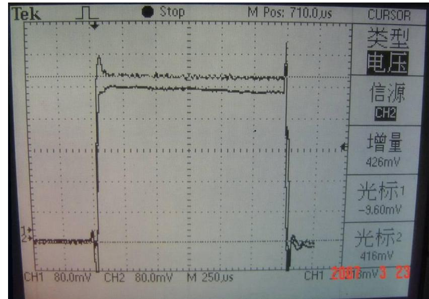
46mA output beam at 7% duty factor, transmission rate > 93%.
