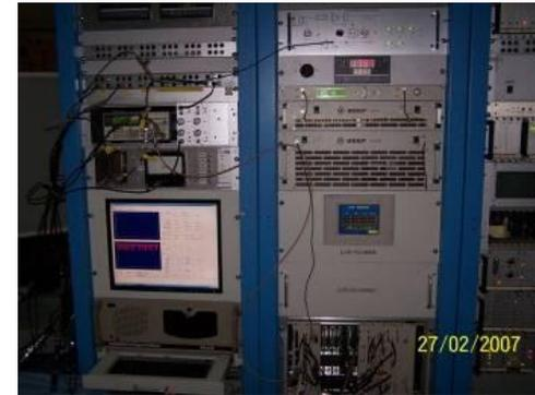
AC resonant HV pulsed power supply for klystron was proposed and devised.
