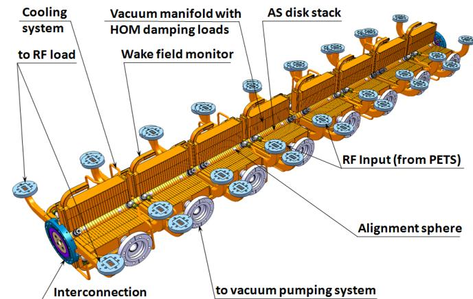
Stack of 8 ac. structures under assembly
