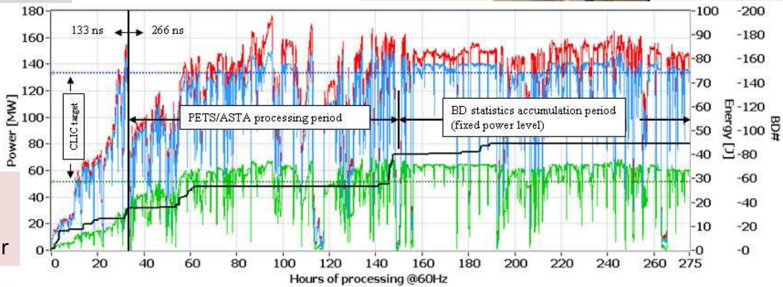
D. Sc No breakdown last  $O(8 \cdot 10^6)$  pulses)  $\rightarrow P$  about consistent with  $p=2.4 \cdot 10^{-7}/m/\text{pulse}$
