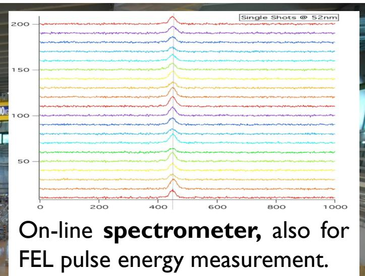
On-line **spectrometer**, also for FEL pulse energy measurement.
