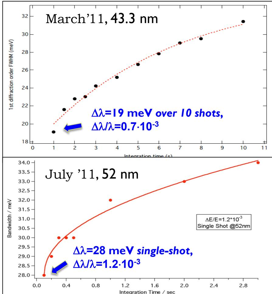
Due to CCD issue, the bw depends on the expos. time. Seed laser:  $\Delta\lambda/\lambda=0.3\%$ ,  $\sim 150\text{fs}$ ,  $\sim 1.2 \text{ FTL}$ ,
