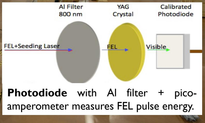
**Photodiode** with Al filter + pico-amperometer measures FEL pulse energy.
