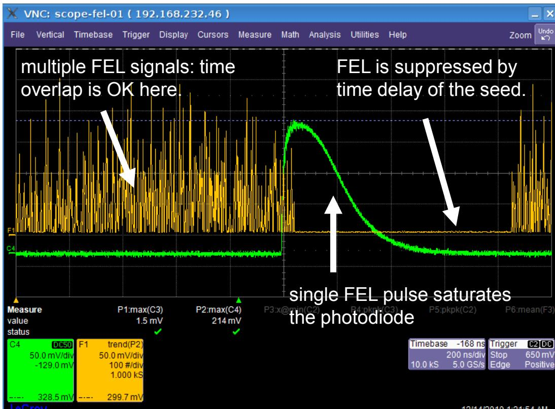
Shot-to-shot signal [a.u.] from atomic photo-ionization of Nitrogen at  $10^{-5}$  mbar.
