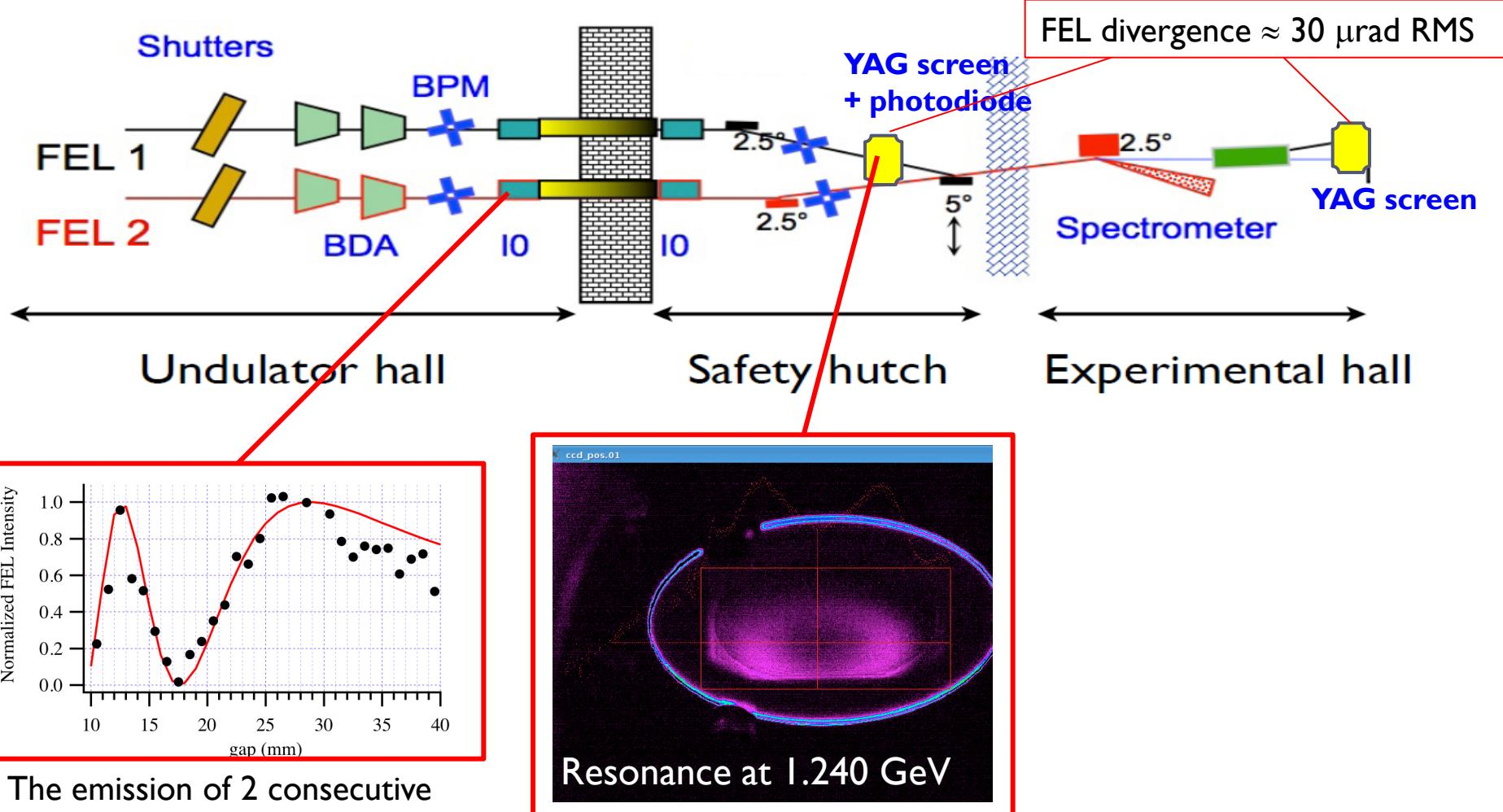
The emission of 2 consecutive radiators tuned at 52 nm sums coherently for a proper gap of the phase shifter. PS calibration and model are confirmed.
