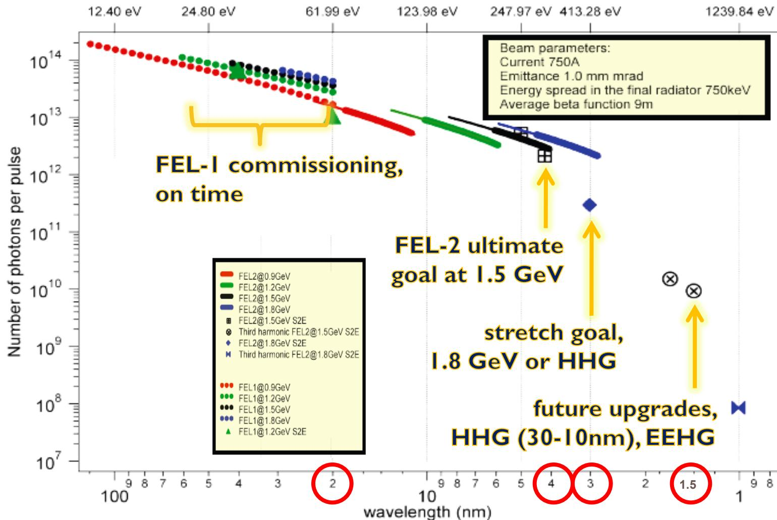
Lines predicted using M.Xie formulae for expected FERMI parameters assuming 40fs pulse length
