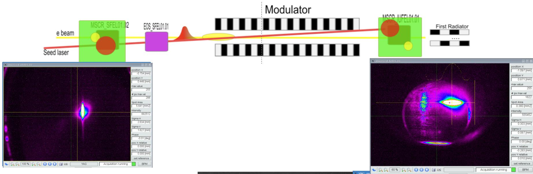
**Time overlap** at the modulator entrance is carried out with an **Al foil** that reflects the laser out of the chamber and makes electrons producing OTR. The two signals are detected with a CCD and a **fast photodiode**. A **delay line** is used for **sub-ps tuning**.
