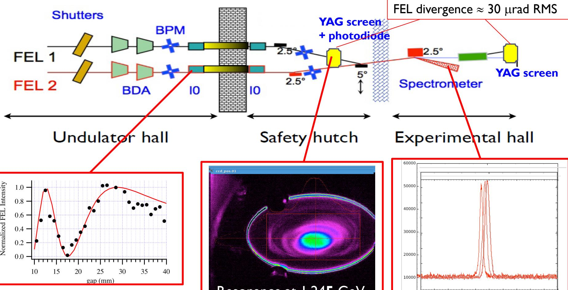
The emission of 2 consecutive radiators tuned at 52 nm sums coherently for a proper gap of the phase shifter. PS calibration and model are confirmed.
