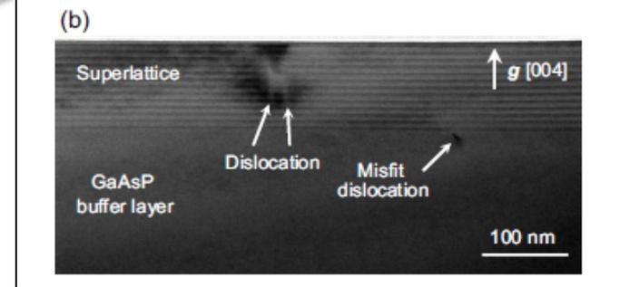
FIG. 2. Cross-sectional TEM images of the GaAsP buffer layer on (a) GaAs, (b) GaP, and (c) a GaP substrate with GaAs IL. Stacking faults are introduced into the GaAsP buffer layer on GaAs, while dislocations are introduced on GaP.
