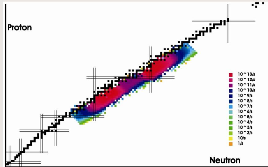
Photo-fission products using 50 MeV 10 mA electrons on to Hg convertor &  $UC_x$  target.
