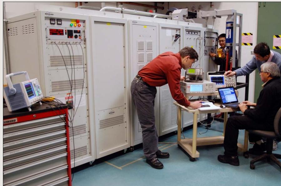
The 30 kW IOT transmitter will be used for the coupler test. Initially rf power will be limited to 10 kW cw for rf conditioning and thermal test of the couplers.
