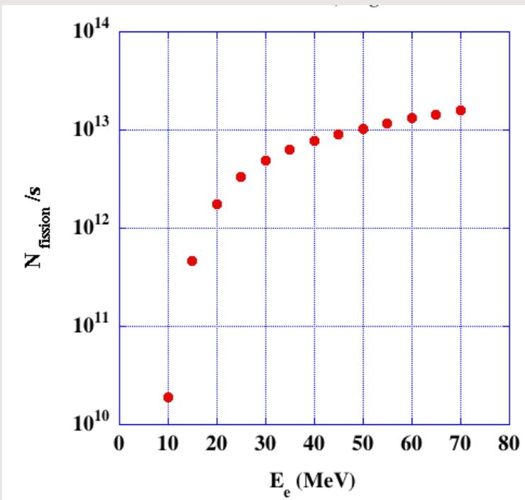
Number of photo-fission/s vs. electron energy for 100 kW e-beam on Ta convertor and U target.
