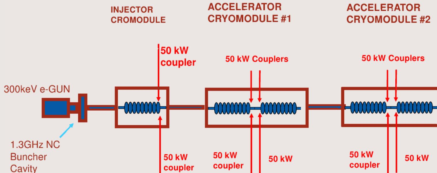
The present e-linac design concept, based on **1.3 GHz Superconducting RF technology (SRF)** in CW operation, offers flexibility, possibility for expansion to other applications (Free Electron Laser, Energy Recovery Linac).
