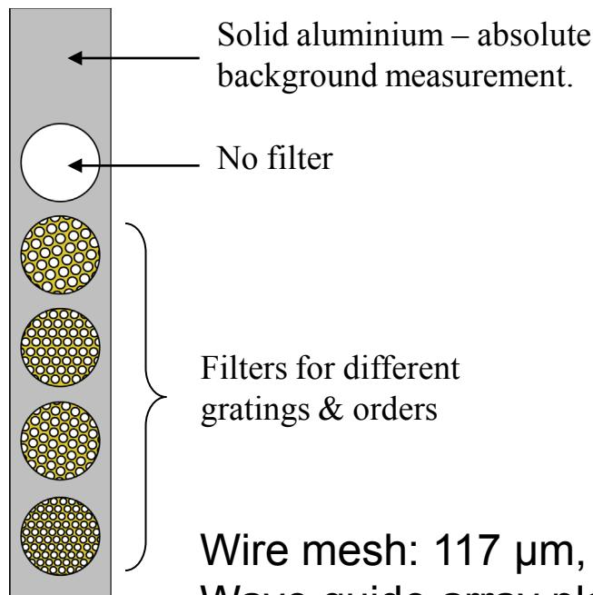
Wire mesh:  $117 \mu\text{m}$ ,  $175 \mu\text{m}$ ;  $\Delta\lambda = 10-20 \mu\text{m}$
