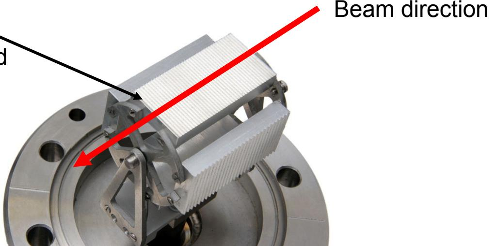
A carousel can rotate and offer three different gratings or one blank to the beam. Rotation is controlled remotely
