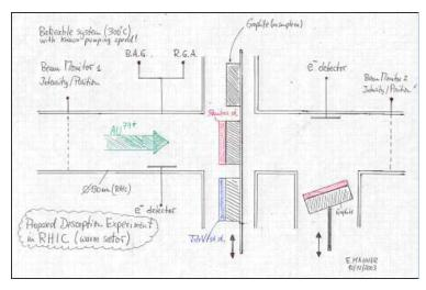
Fig. 2. Proposed RHIC single-pass experiment to measure heavy-ion induced molecular desorption of  $Au^{79+}$  impacting on different targets.
