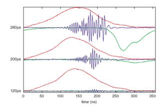
**Fig 1.** Courtesy R.J. Macek. Evolution of the ep instability for a 4.4  $\mu$ C beam. The red trace is the wall current monitor, the blue trace is a vertical beam position monitor difference signal, and the green trace is the electron detector current.
