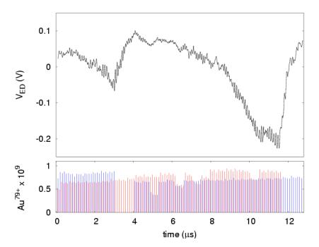
**Fig. 4.** The top plot shows the EC build-up in IR12 during a RHIC revolution (12.8  $\mu$ s). The bottom plot shows the bunch intensity of both blue (blue lines) and yellow (red lines) beams and the relative time position between them. Note a single beam produces a decay in the electron signal (between 2.8 and 4  $\mu$ s – blue abort gap, and 11.6 and 12.8  $\mu$ s – yellow abort gap).
