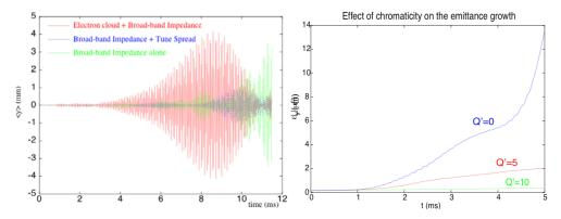
**Fig. 1.** Evolution of the centroid vertical position of an SPS bunch over 500 turns for the three labeled cases (left). Vertical emittance versus time for three different chromaticity settings (right). Broad-band impedance and space charge are included.
