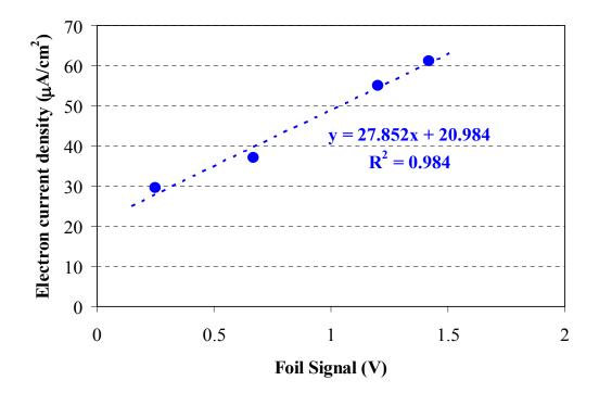
Fig. 9. Effect of varying losses (from foil scattering) on the prompt electron signal in drift section 4 for a beam intensity of 5.8  $\mu$ C/pulse.
