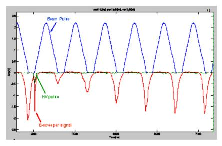
**Fig. 15.** Recovery after sweeping the gap. The red signal is from the electron sweeping diagnostic, the green is the high voltage pulse (500 V) applied to the sweeping electrode and the blue signal is the beam current signal from a wall current monitor (WC41) in the ring.
