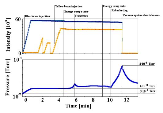
**Fig. 1.** Vacuum instability in Blue sector 8 (unbaked collimators), with 56 bunches per ring. The upper part shows the beam intensities during injection, acceleration and rebucketing. The lower part shows the pressure changes during injection, transition crossing and after rebucketing.
