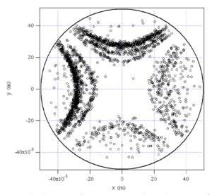
**Fig. 2.** Snapshot of trapped electrons in a PSR quadrupole 5  $\mu$ s after passage of the beam pulse. (Courtesy M. Pivi). As it might be expected, the trapped electrons follow the magnetic field lines.
