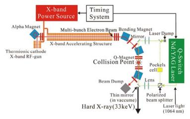
**Fig. 1.** Schematic illustration of Compact Hard X-ray source based on thermionic-cathode Xband RF-gun, X-band accelerating structure and Q-switch Nd:YAG laser with laser light circulation system.
