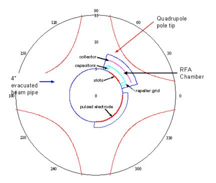
Fig. 23. Schematic layout of a proposed electron sweeping diagnostic in a PSR quadrupole.
