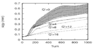
Fig. 2. Vertical rms-size growth of a KEK bunch for different values of the chromaticity (labelled in  $Q' = \xi_y Q_y$ )
