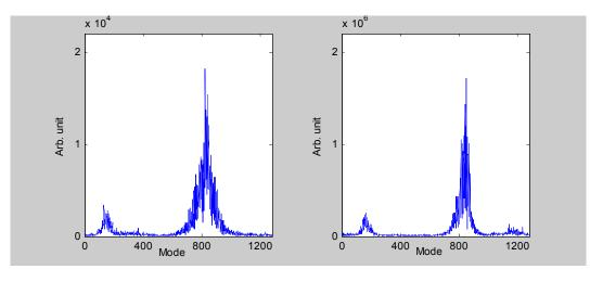
Fig. 4. Horizontal mode spectrum Fig. 5. Vertical mode spectrum [without solenoid field]
