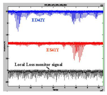
**Fig. 16.** Multi-turn (110) sequence of signals from two electron detectors (ES41Y and ED42Y) and a local loss monitor in section 4 of the ring.
