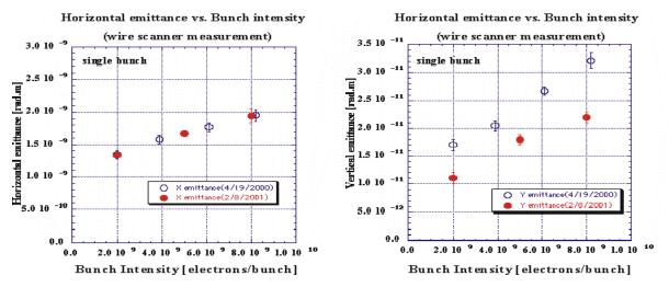
Fig. 2: Recent results of emittance measurements using wire scanners at the EXT.
