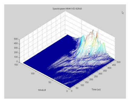
Fig. 22. Spectrogram of the BPM signal collected for a 5  $\mu$ C/pulse unstable beam. The time origin is the end of injection. The vertical axis is the fft amplitude of the BPM signal.
