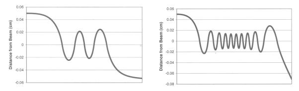
**Fig 6.** For 40-ps-long (12-mm) positron APS bunches, electrons that are within about 500  $\mu$ m of the beam center oscillate several times in the bunch potential (calculations are for vertical plane). The bunch current is 2 mA on the left, 10 mA on the right. The transverse rms beam size is 350  $\mu$ m (horizontal) and 50  $\mu$ m (vertical).
