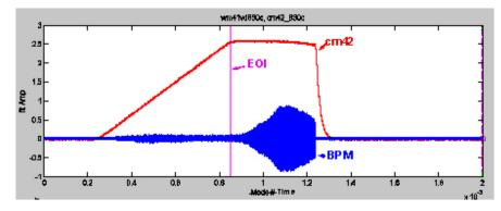
**Fig. 20.** Beam response to a weak one-turn vertical kick applied at the end of injection (EOI). The blue trace is the vertical difference signal from a stripline BPM and the red trace is current monitor (CM42) showing the stored current in the ring during accumulation and a 500 µs store.
