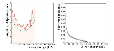
**Fig. 2.** Energy spectrum and energy (left figure ) vs. scattering angle (right figure) of X-ray in single bunch(20pC/bunch) collision with Q-switch Nd:YAG-laser(2J/pulse). Scattering angle of 0 rad is direction of electron beam.
