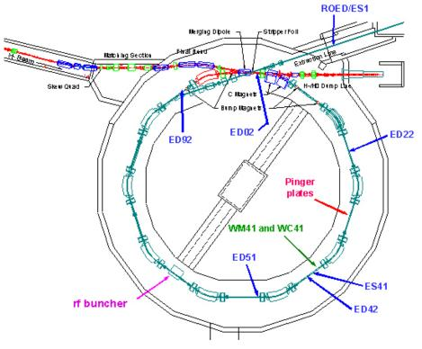
Fig. 24. PSR layout including electron detectors and e-p diagnostics.
