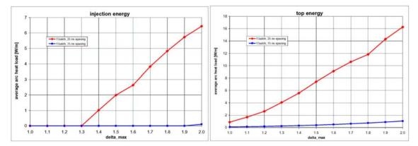
**Fig. 2:** Simulated average arc heat load as a function of the maximum secondary emission yield for bunch spacings of 25 ns and 75 ns at injection (left) and at top energy (right).
