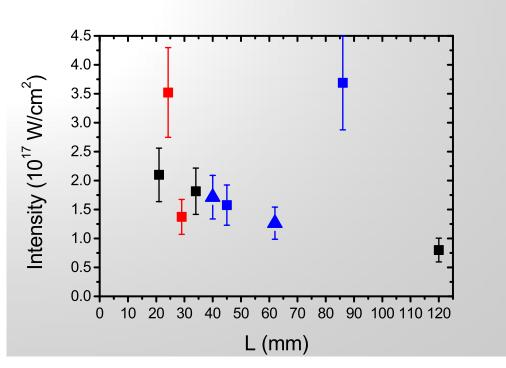
**Fig. 3:** Intensity as a function of the capillary tube length for different capillary tube radii: 25  $\mu$ m (black squares), 35  $\mu$ m (red squares) and 38  $\mu$ m (blue squares) in vacuum; on some shots the capillary tubes were filled with 2.2 mbar of helium gas (38  $\mu$ m radius, blue triangles).
