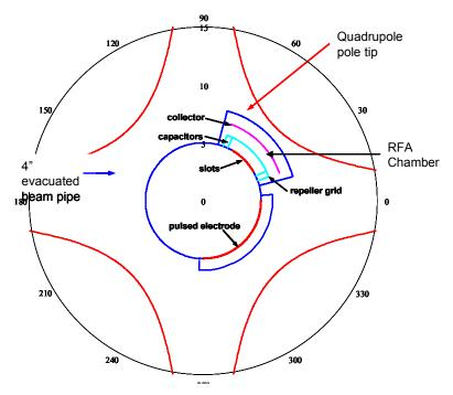
Fig. 3. Schematic cross section of a proposed electron sweeping detector for a PSR quadrupole.
