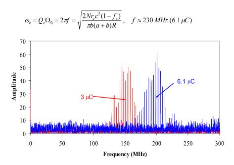
Fig. 1. Plot showing the spectra of betatron sidebands from a stripline BPM (vertical difference signal) taken during unstable motion near threshold for two different intensities (6.1 and 3  $\mu$ C/pulse respectively).
