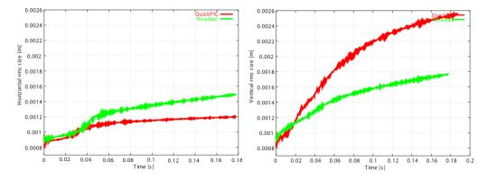
**Fig. 4.** Horizontal (left) and vertical (right) emittance growth in LHC. The green lines are simulations done with HEADTAIL, the red lines correspond to QuickPIC simulations (with the 1-kick approximation). All simulations are carried out with conducting boundary conditions on a rectangular beam pipe.
