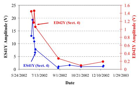
**Fig. 14.** Plot showing the reduction of the prompt electron signal amplitudes for two RFAs (ED42Y and ES41Y in section 4 of the ring) during 2002 operations.
