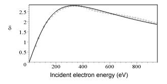
Fig 4. Measured  $\delta$  for Al APS chambers, fitted to empirical formula in Ref. [8].
