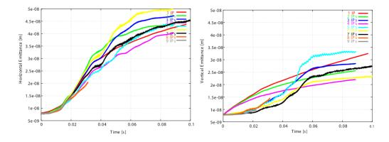
**Fig. 3.** Horizontal (left) and vertical (right) emittance growth in LHC as function of the interaction points used in the simulation.
