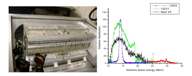
**Fig. 2.** Inverse free-electron laser undulator at Neptune laboratory (left); measured momentum spectra from selected shots, showing no laser, 5 MeV energy gain, up to 15 MeV acceleration (right).
