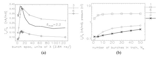
**Fig 3.** Electron beam: (a) Measured (RFA 3,6) and simulated (dashed line) wall current vs. bunch spacing. There is additional conditioning of 100 Ah for these data compared to Fig. 2a, main plot. (b) Measured wall current as a function of bunch train length. The signal near EA (RFA 1) is always higher than RFA 6. No anomalous pressure rise is observed.
