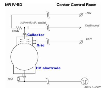
Fig. 1. Electron sweeping detector at the KEK-PS Main Ring.
