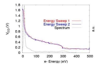
**Fig. 2.** The red and blue traces show the electron signal in the ED when filtering the electron energy from 0 to 500 eV. The corresponding differentiated spectrum is shown by the black trace. Note that the noise in the ED is about 0.15 V.
