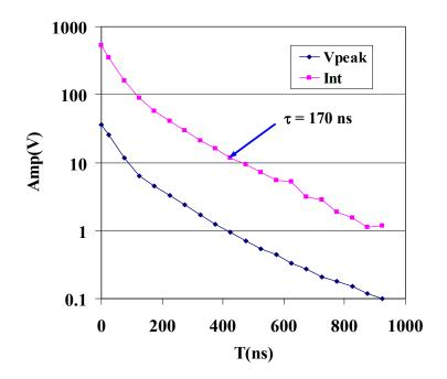
Fig. 6. Electron dissipation as measured with the electron sweeping diagnostic.
