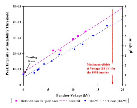
**Fig. 2.** Plot of threshold intensity as a function of rf Buncher Voltage. The square points are historical data for operational beams prior to the direct H<sup>-</sup> injection upgrade in 1998 and the blue circles in Oct 1998 after the upgrade.
