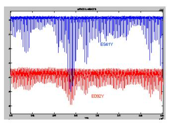
**Fig. 17.** Multi-turn (~100) sequence of signals from two electron detectors (ES41Y and ED92Y) located in section 4 and section 9 respectively.
