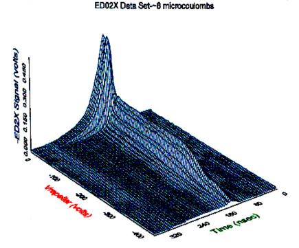
**Fig. 4.** The three-dimensional plot of RFA signals as a function of time and repeller voltage shown here provides a cumulative energy distribution of electrons striking the wall.
