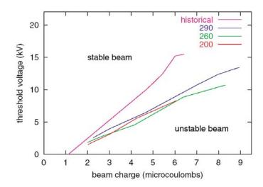
**Fig 2.** Courtesy R.J. Macek. Threshold RF voltage versus beam charge. The historical curve represents the situation before the direct H- injection upgrade. Threshold curves near the end of the extended 2001 run for injected bunch lengths of 200, 260, and 290 ns. are shown for comparison.
