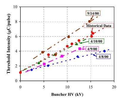
**Fig. 12.** Threshold intensity curves showing the benefit of beam conditioning (scrubbing) during 2000 when there were no inductive inserts in PSR.
