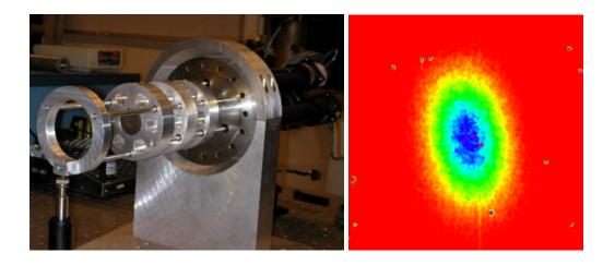
**Fig. 3.** UCLA-built adjustable strength PMQ triplet, with >500 T/m Halbach quads (left); X-ray CCD image of inverse-Compton shot at PLEIADES with  $\sim 2 \times 10^6$  photons — this number is expected to rise by an order of magnitude with the PMQ final focus (right).
