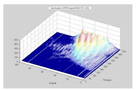
**Fig. 21.** Spectrogram of the BPM signal from the beam response to a weak kick. The origin of the time axis is the time of application of the one-turn kick. The vertical axis is the fft amplitude of the BPM signal.
