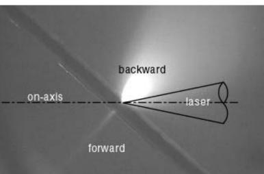
**Fig. 2 :** Photograph taken at the moment of laser irradiation to an Al foil of 3 m in thickness. A laser is coming from the right side. The target foil is tilted by 45 degrees with respect to the laser axis.
