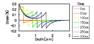
**Fig. 6.** The strain wave propagation into a GaAs crystal.
