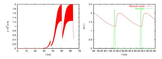
**Fig. 9.** Electron cloud build up in an IR in RHIC (left) and with bunch structure in the saturation regime (right)
