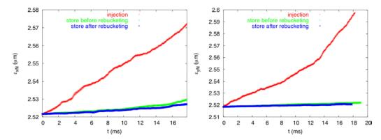
**Fig. 8.** Horizontal (left) and vertical (right) normalized emittance growth for a Au<sup>79+</sup> bunch in RHIC at injection (red), at top energy before rebucketing (green) and at top energy after rebucketing (blue). The electron cloud density is  $10^{12}$  m<sup>-3</sup>
