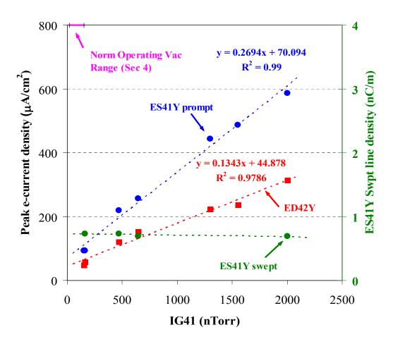
**Fig. 11.** Prompt electron signals (ES41Y and ED42Y) plus the swept electron signal at the end of the gap (ES41Y swept) are plotted as a function of the vacuum pressure in section 4. Beam intensity was 8.2  $\mu$ C/pulse (5x10<sup>13</sup> protons per pulse).
