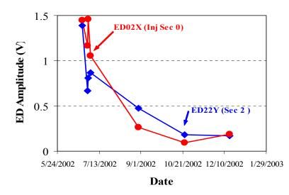
**Fig. 13.** Plot showing the reduction of the prompt electron signal amplitudes for two RFAs (ED02X and ED22Y) during 2002 operations.
