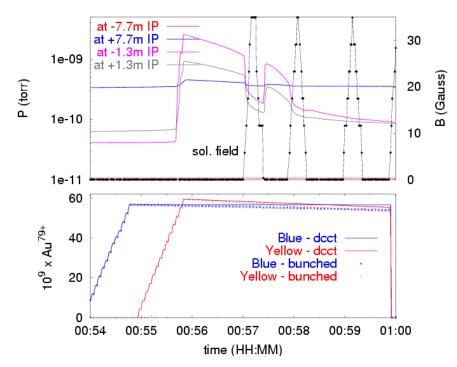
**Fig. 3a.** Pressure rise (top plot) while injecting 56 bunches in each ring, spaced by 216 ns (bottom plot) in fill 4791. Note that weak solenoid fields (around 10 Gauss) decrease the pressure value by a factor of 10.
