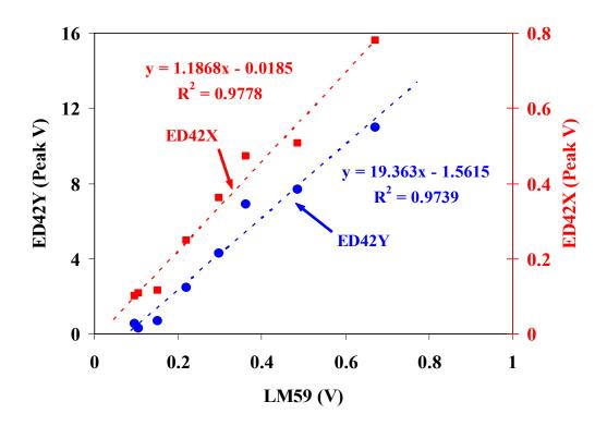
**Fig. 10.** Prompt electron signals from ED42X (detector in the horizontal plane) and ED42Y (detector in the vertical plane) plotted against the variation of local losses produced by horizontal closed orbit bumps in section 4 of PSR. The beam intensity was 8.1  $\mu$ C/pulse (5x10<sup>13</sup> protons per pulse).
