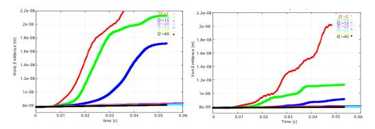
Fig. 5. Horizontal (left) and vertical (right) emittance growth in LHC for different chromaticity values and  $\rho_e = 6 \times 10^{11} \text{ m}^{-3}$ , simulated by HEADTAIL.
