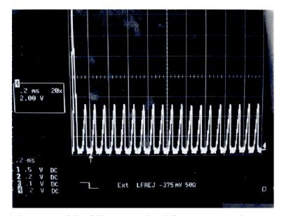
**Fig. 19.** Sequential capture of the foil current signal for 20 consecutive macro pulses after a several minute beam off time.
