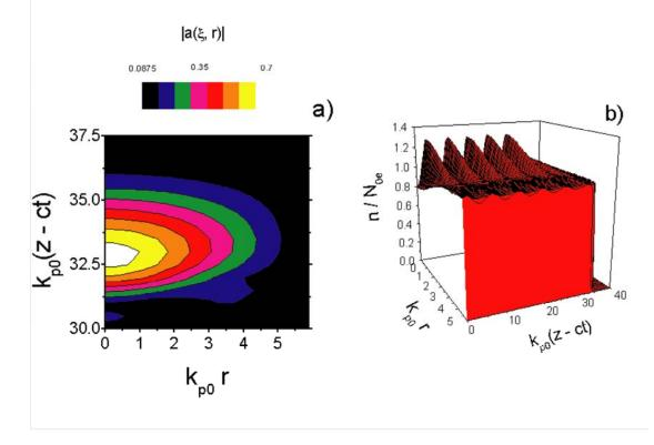
**Fig. 1:** a) Contour plots of the laser pulse envelope  $|a(\xi, r)|$  in the  $(\xi, r)$  plane and b) normalized electron plasma density  $n(\xi, r)/N_{0e}$  at the propagation distance from the entrance of the capillary tube z = 4.61 cm for a hydrogen filled capillary tube.
