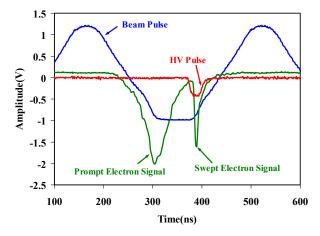
Fig. 5. Signal from the electron sweeping diagnostic.
