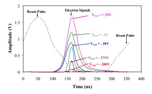
Fig. 3. Examples of electrons signals observed with an RFA shown in time relation to the beam.
