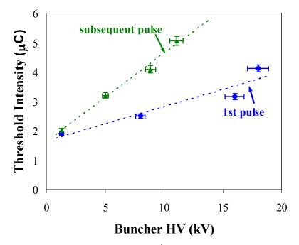
**Fig. 18.** Instability threshold curves for the 1<sup>st</sup> unstable pulse (blue) and subsequent pulses (green).
