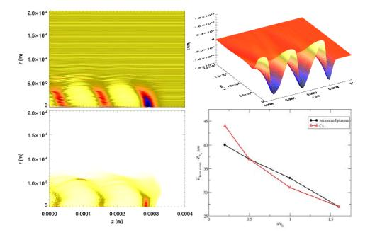
**Fig. 2.** Electron density contours for the case of 100% pre-ionized plasma (top left) and tunneling ionization of Cs by the e+ beam (bottom left), which yield amazingly similar wakefields (top right). The optimal distance from e+ drive beam to witness beam  $[\mu m]$  is shown (bottom right) vs Cs gas density, normalized to the prediction of Eq. (2).
