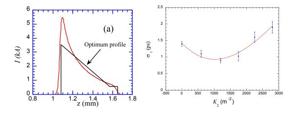
**Fig. 4.** Ramped beam profile expected after sextupole correct in Neptune dogleg compressor, for enhancement of plasma wakefield transformer ratio (left); Sextupole correction giving minimum pulse length, as measured using CTR at Neptune (right).
