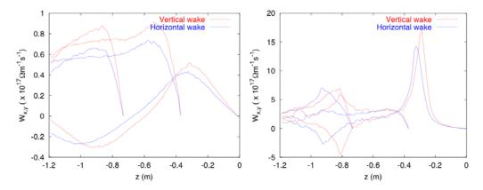
**Fig. 6.** Horizontal and vertical averaged dipole wake functions (left) or wake functions on axis (right) for an SPS bunch. They have been evaluated displacing three different bunch slices at t=0,  $3/10 \Delta t_b$ ,  $3/5 \Delta t_b$ .
