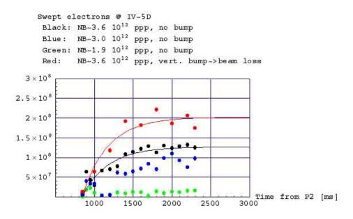
Fig. 5. Number of electrons swept out with HV ( $\sim -850$  V, 100 ns) after a time from the acceleration starting trigger. RF is turned off at  $\sim 850$  ms.
