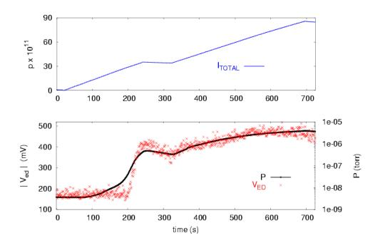
**Fig. 1.** The top figure shows the total beam current injected in RHIC. Note that injection was temporally interrupted after injection of 45 bunches (t=250 s), and resumed at t=320 s. The bottom picture shows the pressure evolution (black line) and the voltage (absolute value) in the ED (red crosses) while this injection takes place. The noise in the ED is about 150 mV.
