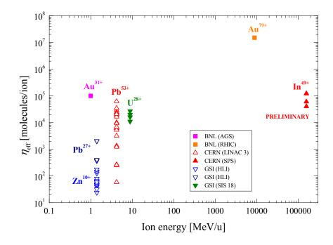
**Fig. 1.** Overview of heavy-ion induced desorption data, obtained at BNL [1, 2], CERN [3, 4, 5], and GSI [6, 7]. The ion impact angles (perpendicular, mrad,  $\mu$ rad) of the experiments are different (see text).
