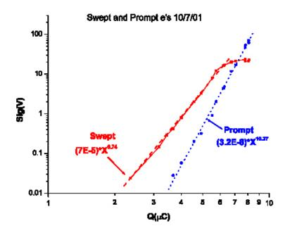
**Fig. 7.** Prompt and swept electrons signal amplitudes plotted as functions of beam intensity (Q).
