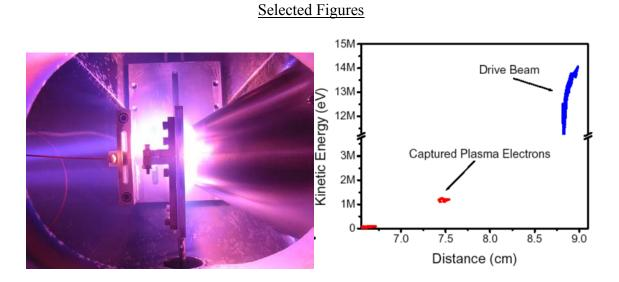
**Fig. 1.** Plasma source for UCLA/NICADD trapping injection experiment at FNAL A0 (left); simulated longitudinal phase space from experiment, from MAGIC code (right).
