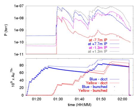
**Fig. 3b.** Pressure rise in the different gauges of IR12 while injecting 110 bunches in each ring, spaced by 108 ns (fill 4794). In this case, the pressure only decayed by a factor of 2 when applying solenoid fields.
