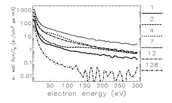
**Fig 5.** Energy distributions from differentiated RFA signals as a function of bunch spacing (units of  $\lambda$ ) (10 bunches, 2 mA/bunch). Low-energy part is well fit by a Lorentzian with  $\langle E \rangle 2.5$  eV and width 4 eV. There is a long exponential tail on all but 128  $\lambda$ . Energy bumps are observed for 2  $\lambda$  and 4  $\lambda$ , but not on longest tail for 7  $\lambda$ .
