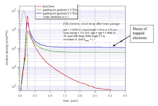
**Fig. 1.** Simulations of electrons in a PSR quadrupole. (Courtesy M. Pivi). The red curve is the simulated electron density in a field free region, the green curve is the electron density for the standard-gradient quadrupole (3.9 T/m) in the PSR and the blue curve for a gradient of 8.5 T/m. Note the very slow decay of electrons trapped in the quadrupole long after the beam pulse has passed.
