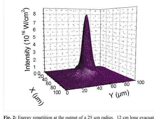
Fig. 2: Energy repartition at the output of a 25  $\mu$ m radius, 12 cm long evacuated capillary tube for an incident energy in the focal plane of 4.3 J.
