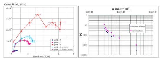
**Fig. 3:** Electron volume density simulated by ECLOUD as a function of average-arc heat load at top energy (left) and emittance growth rise time simulated by HEADTAIL as a function of electron volume density at injection (right).
