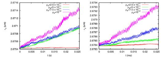
**Fig. 7.** Horizontal (left) and vertical (right) emittance growth for a long Au<sup>79+</sup> bunch in RHIC and different integrated electron cloud densities.
