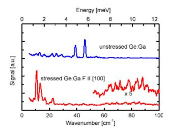
Figure 3: Photoconductivity spectra of unstressed and stressed Ge:Ga.
