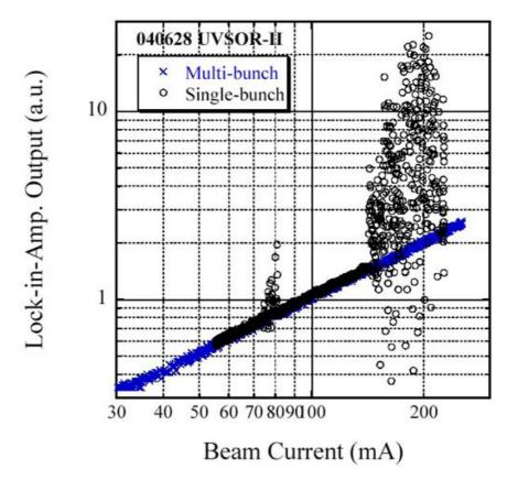
**Figure 1:** Intensity of the terahertz radiation observed at the infrared beam line BL6B of UVSOR-II. The blue crosses are the data taken in multi-bunch mode and the white circles in single bunch mode. The chopper frequency was 100Hz.
