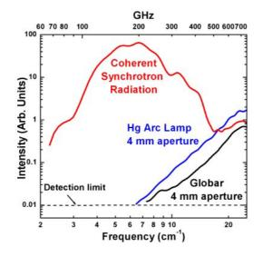
**Figure 1:** Measured far-IR intensity for the BESSY CSR source, compared to mercury arc and tungsten conventional thermal sources. While the turn-on of the CSR source below 2 cm<sup>-1</sup> is a real effect of the CSR emission process, the drop off at the low frequency end is due to a combination of diffraction losses in the optical path of the beamline and the cutoffs of the optical components, such as the mylar beamsplitter, in the interferometer.
