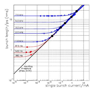
Figure 7: Measured bunch lengths as a function of the current, indicated by coloured dots. Blue: streak camera data and empirical fit to the data; black: bursting threshold of coherent THz signals; red: coherent THz radiation based data. At the fitted data lines the  $f_s$  values are indicated.
