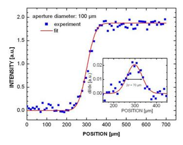
Figure 10: Measured and fitted spatial resolution curves for an exit aperture of  $100 \,\mu m$  diameter. The inset shows a Gaussian fit of the first derivative of the measured curve used to determine the spatial resolution.
