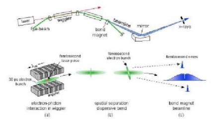
**Figure 4** Schematic of laser slicing of an electron beam. The beam energy is modulated via interaction with a laser pulse in a wiggler. The energy modulation leaves a hole in the bunch via time-of-flight dispersion of the modulated beam. The "hole" can then radiate coherently.
