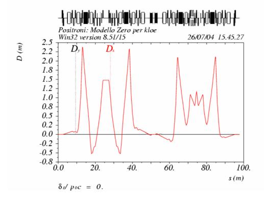
Figure 9: Dispersion function along the ring with wigglers ON.
