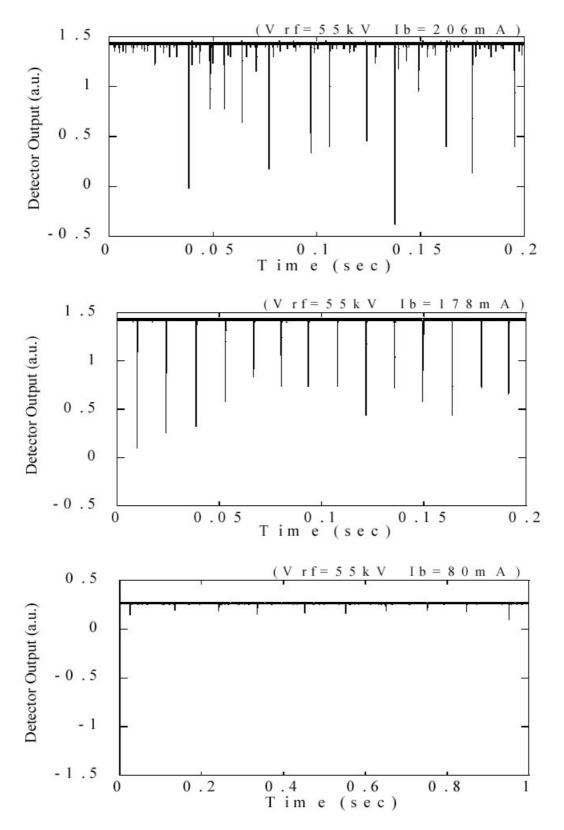
**Figure 2:** Terahertz bursts at three beam currents, 206mA (top), 178 mA (middle) and 80 mA (bottom). The output signal (negative) of the bolometer was recorded with a digital oscilloscope. The bursts appear chaotically at the higher beam current and quasi-periodically at the lower beam current. The horizontal scale in the lowest figure is larger than others.
