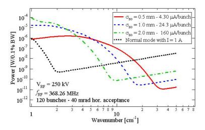
Figure 3: Calculated SR Spectra for three different sets of DA $\Phi$ NE as ultra-stable source of CSR.
