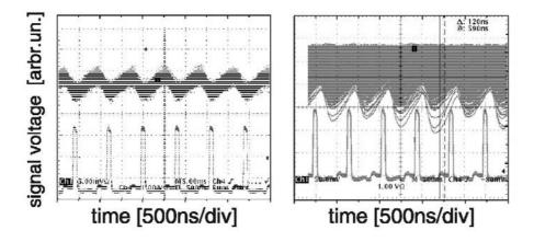
**Figure 4:** THz-signals of stable (left, upper part) and bursting CSR (right, upper part) together with the beam revolution trigger (lower part) in time domain. The stable CSR shows a sawtooth-like, periodic signal, of constant amplitude. The bursting CSR shows a stochastic distribution of signal amplitude. The detector is of InSb with 1 MHz bandwidth, which resolves the bunch revolution in the storage ring of 1.25 MHz.
