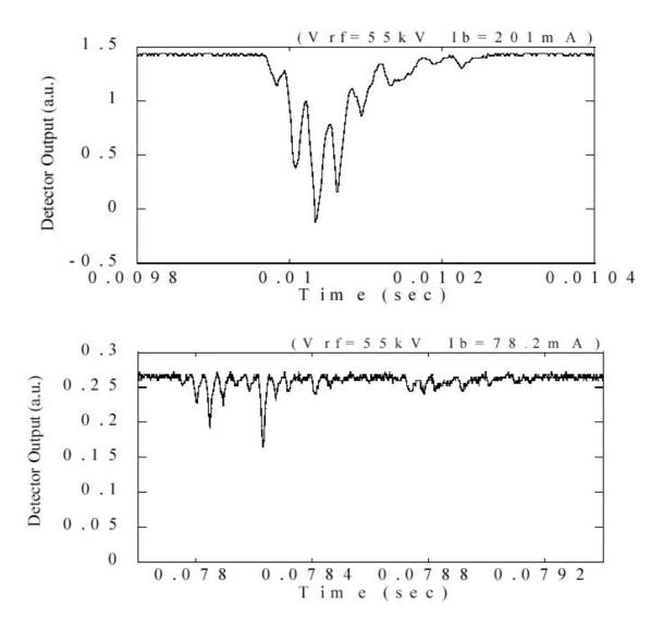
**Figure 3:** Some examples of the temporal profiles of the individual bursts at the beam current of 201mA (upper) and 78mA (lower). The output signal (negative) of the bolometer was recorded with a digital oscilloscope.
