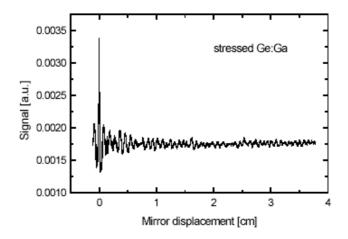
Figure 2: Interferogram obtained from the stressed Ge:Ga crystal
