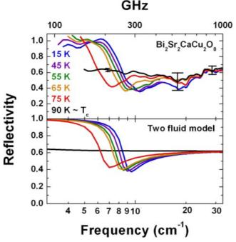
**Figure 5:** Measured c-axis polarized near-normal reflectivity of  $Bi_2Sr_2CaCu_2O_8$  (upper panel) for various temperatures at or below the superconducting transition temperature,  $T_c$ . A resonance that shifts with temperature and disappears above  $T_c$  is clearly observed. The lower panel shows the calculated reflectivity of a superconductor with a shifting Josephson Plasma Resonance.
