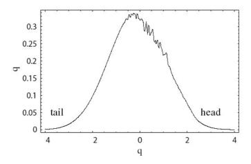
Figure 5: Bunch density with "microbunching"
