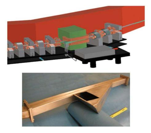
**Figure 2**. Top) Cutaway view of a dipole source with optical table. The experiment sits less than 1 m from the source of the radiation. Bottom) A photograph of a full-scale prototype chamber fabricated for RF testing. The chamber is designed to collect 300 mrad horizontally and 140 mrad vertically. This very large acceptance means that the first mirror collects 95% of the radiation at 1 mm wavelength, so the CSR extraction is very efficient.
