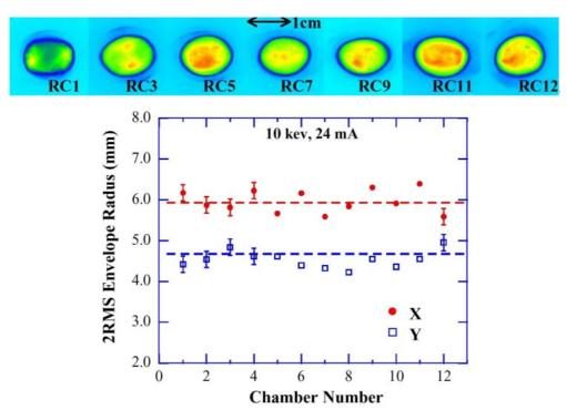
**Figure 4**: False color rendering of beam pictures at 7 of 12 ring chambers (top), and measured 2rms beam dimensions (X: horizontal, Y: vertical) vs. calculated values represented by dashed lines (bottom). The distance between chambers is 64 cm.
