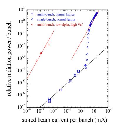
**Figure 2:** Radiation power vs. stored beam current per bunch in three cases; (1) and (2) normal alpha and (3) low alpha. The red lines and black line are guides which indicate the expected dependences when the power is proportional to the square of the current (CSR) or simply to the current (incoherent SR).
