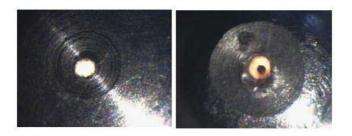
**Figure 8:** Aperture of 200  $\mu$ m diameter with a coaxial wire of 80  $\mu$ m thickness (right) and without a wire left).
