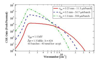
**Figure 7**: Calculated CSR gain for the three different sets of DA $\Phi$ NE with the superconductive RF system. The curves have been obtained dividing the power spectra by the spectrum of DA $\Phi$ NE in the normal operation mode with 1 A stored.
