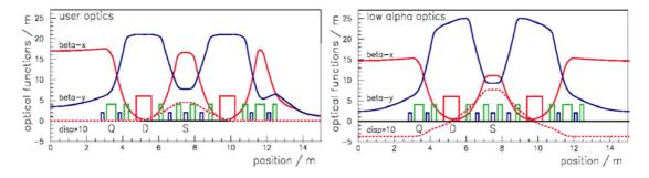
**Figure 1:** Optical functions of the user (left) and the low alpha optics (right) of one out of 16 ring cells. Dipoles, quadrupoles and sextupoles are indicated by D, Q and S, respectively.
