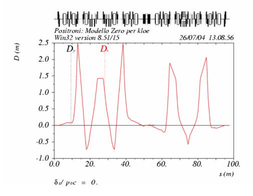
Figure 11: Dispersion function along the ring with wigglers OFF.
