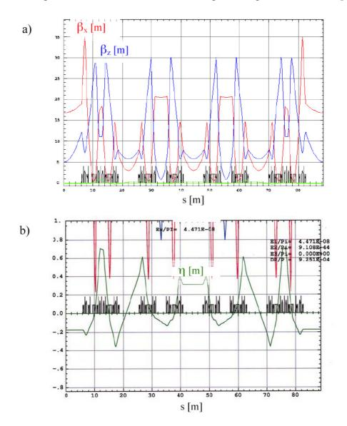
**Figure 1:** SOLEIL lattice functions in the mode with low first-order momentum compaction factor: (a) horizontal and vertical beta-functions and (b) horizontal dispersion function.
