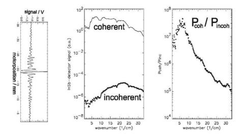
**Figure 5:** The left figure shows an example of an autocorrelation function of coherent emission. The figure in the middle shows the measured spectra of the coherent and incoherent case at equal bunch current, without any correction. The right figure shows the ratio of the two spectra, yielding the power spectrum times the number of particles, ranging from about 3 1/cm to 30
