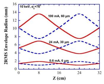
**Figure 3**: Calculated matched rms envelopes in one FODO period of UMER for  $\sigma_0=76^0$  (zero-current phase advance per period). For comparison, the vacuum pipe radius is 25.4 mm.
