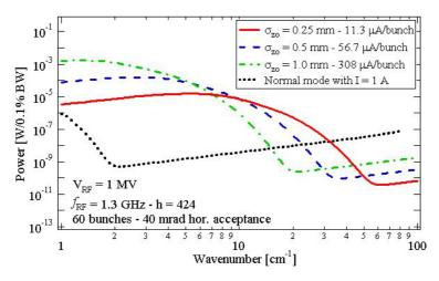
Figure 6: Calculated SR Spectra for the three different sets of  $DA\Phi NE$  with the superconductive RF system.
