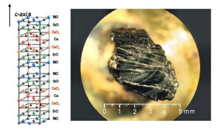
**Figure 4:** Structure of  $Bi_2Sr_2CaCu_2O_8$  (left) and the mosaic of the single crystals used in this investigation (right). To account the contribution to the measured reflectance the area of epoxy showing was estimated and the experimental reflectance was corrected accordingly.
