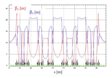
**Figure 3:** SOLEIL lattice providing large vertical beta-function in straight sections occupied by RF cavities.
