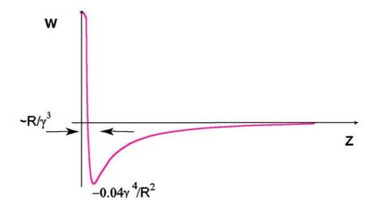
Figure 1: CSR wake as a function of distance. A simple formula (3) is applicable for not very short distances, to the right of the minimum of the wake. The wake reaches minimum at  $z \sim R/\gamma^3$ , with the minimum value of  $-0.04\gamma^4/R^2$ .
