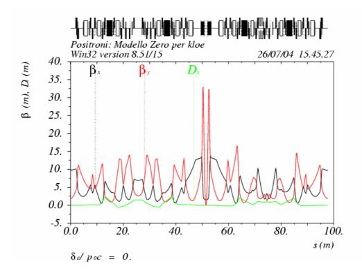
Figure 8: Betatron functions along the ring with wigglers ON.
