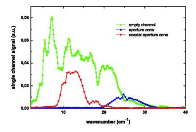
**Figure 9:** Single channel spectra of the empty spectrometer channel, of the aperture cone and of the coaxial aperture cone. The intensity of the empty channel spectra is attenuated by a factor of 100. Note, that the single channel intensities are shown in a linear scale. Intensities through both cones are for wavenumbers down to  $2 \text{ cm}^{-1}$ .
