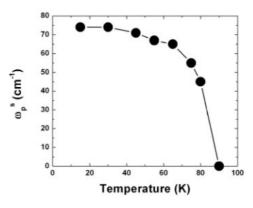
**Figure 6:** Superfluid plasma frequency as a function of temperature. Plasma frequency was determined from fitting the reflectance spectra with the two fluid model shown in the bottom panel of Figure 5.
