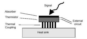
Figure 1: Schematic of a bolometric detector.
