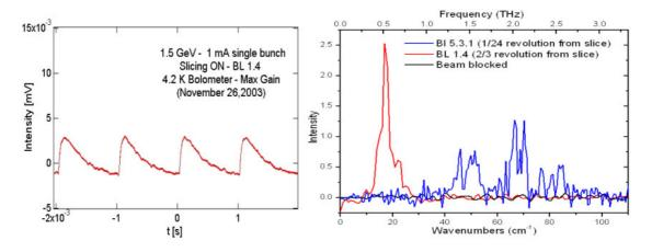
**Figure 6**: Left) The infrared signal measured with the nominal lattice at the BL1.4 with laser turned on and electron bunch current of  $\sim 1$  mA. Right) Spectra measured at BL 5.3.1. and BL1.4. The structure on the measurement is due to reflections in the beam line and water vapor absorption.
