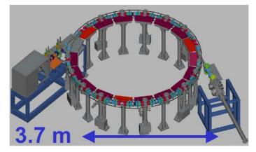
**Figure 1**: University of Maryland Electron Ring photograph (top) and final future layout (bottom) with extraction section on the right-hand side.
