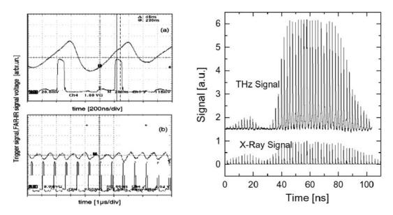
**Figure 5:** Fill pattern measured with an InSb detector (left, upper trace: InSb signal, lower trace: trigger signal, from [2]) and a superconducting NbN HEB (right, lower trace: x-ray signal measured with APD). Note the different time scales: only the NbN HEB allows to resolve single bunches.
