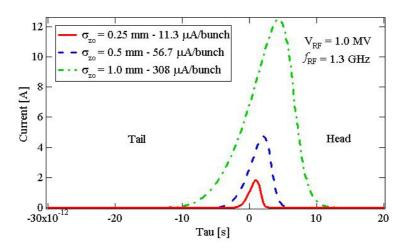
**Figure 5**: Calculated longitudinal distribution of the bunch for the three different modes of  $DA\Phi NE$  with the superconductive RF system.
