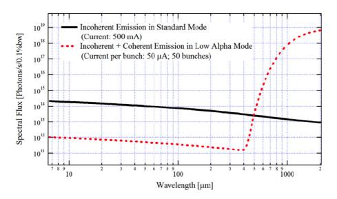
Figure 2: The estimated incoherent and coherent SR spectral flux through the SOLEIL IR extraction port..
