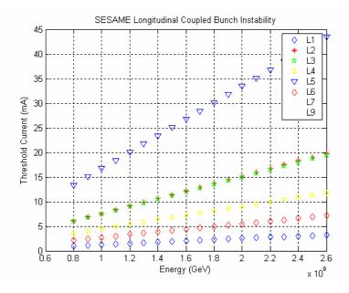
Figure 4: Threshold current due to HOMs versus energy
