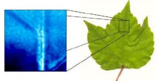
**Figure 11:** Near-field THz image (left) of a section of a *parthenocissus* leaf. Less absorption is indicated by a darker region in the THz image.
