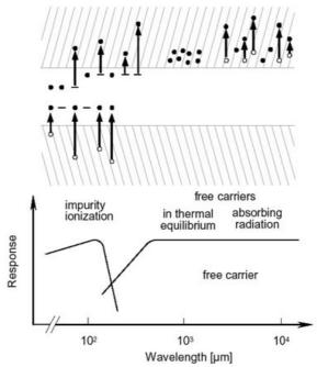
**Figure 2:** Detection mechanisms of a photoconductive detector (impurity ionization) and an InSb hot electron bolometer (free carrier absorption) (after [6]).
