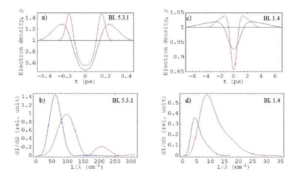
**Figure 5**: A predicted perturbation in the electron density distribution and a spectrum of the infrared radiation caused by this perturbation shown for BL5.3.1 and BL1.4 for the nominal lattice (red line) and for the experimental lattice with an increased momentum compaction factor (blue line). Plots a) and c) show the distribution and plots b) and d) show the corresponding spectrum.
