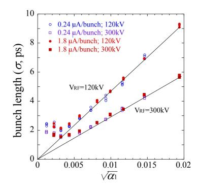
**Figure 1**: Bunch length vs.  $\sqrt{\alpha_1}$ . The symbols are measured length and the lines are theoretical calculation. The RF acceleration voltage was kept constant at 120kV or 300kV while changing  $\alpha_1$ . The open symbols and the shaded symbols are the results with stored beam current of 1.8 and 0.24  $\mu$ A/bunch, respectively. The resolution of the camera was not corrected.
