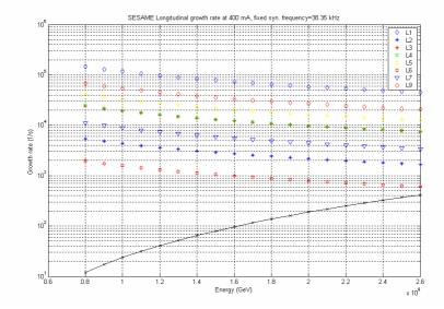
Figure 3: Growth rate (1/s) versus energy for the cavity HOMs
