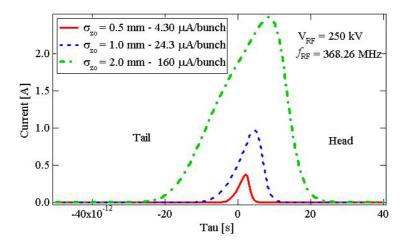
**Figure 2**: Calculated longitudinal distribution of the bunch for three different modes of DAΦNE as ultra-stable source of CSR.
