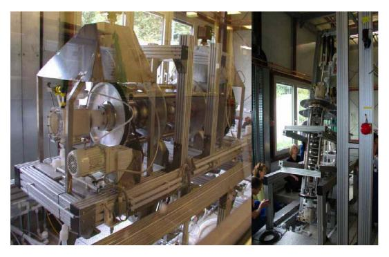
Figure 3: Electro polishing setup at DESY.
