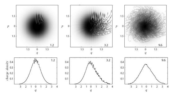
**Figure 6**: Time evolution of bunch under effect of CSR in a compact storage ring. Density plots in phase space (top row) and charge density (second row). Pictures are taken at (normalized) time  $\tau = 1.2$ , 3.2, and 9.6. Instability initiated by a small perturbation with mode number n = 702 (wavelength  $\lambda = 2.2$  mm). A unit of q corresponds to 1 cm.
