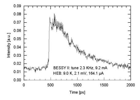
**Figure 6:** Emission of a single electron bunch measured by a NbN HEB. The length is due to multiple reflections in the beamline.
