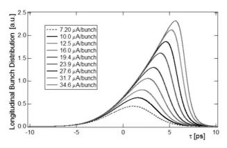
**Figure 5**: Example of calculated bunch distributions for the case of the free space SR wake and positive momentum compaction.
