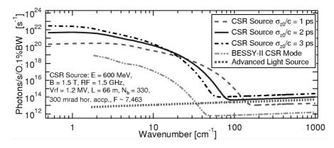
**Figure 7**. Example of source optimized for the CSR production using the criteria described in this paper. The photon flux is compared with the cases of a conventional SR source (ALS) and of BESSY II CSR mode with 400 bunches, 19.2  $\mu$ A/bunch,  $\sigma_{z0}/c = 1.8$  ps and 60 mrad horizontal acceptance.
