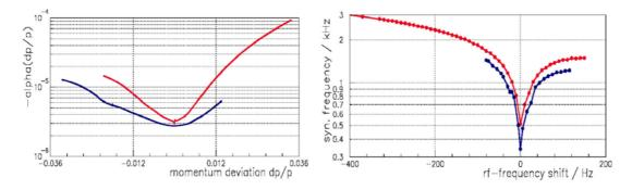
Figure 2: The right part of the figure shows two measurements of the dipole mode of the synchrotron frequency  $f_s$  as a function of the rf-frequency for an optics with  $-\alpha_0 < 10^{-5}$ . From this measurements  $\alpha$  as a function of the momentum was derived, left part of the figure (vertical axis shows - $\alpha$ ).
