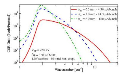
**Figure 4.** Calculated CSR gain for the three different sets of DA $\Phi$ NE as ultra-stable source of CSR. The curves have been obtained dividing the power spectra by the spectrum of DA $\Phi$ NE in the normal operation mode with 1 A stored.
