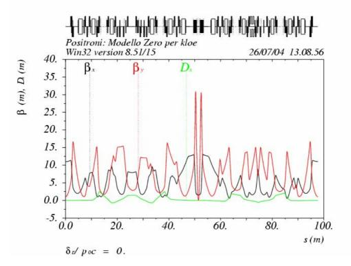
Figure 10: Betatron functions along the ring with wigglers OFF.
