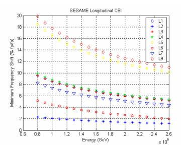
Figure 5: Minimum related frequency shift versus energy
