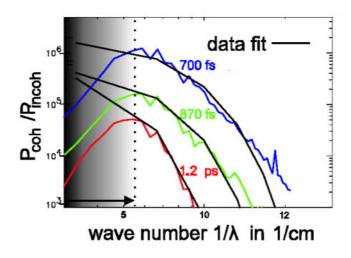
**Figure 6:** Power spectra of different bunches. The bunch lengths are fitted by simulations, using bunches of 700 fs at 0.3  $\mu$ A, 870 fs at 0.14 $\mu$ A and 1.2 ps at 0.14  $\mu$ A rms length. Transmission limitations of the diagnostic system become apparent below 6 1/cm.
