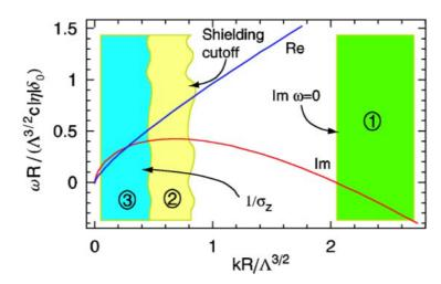
**Figure 2**: Plot of real (blue) and imaginary (red) parts of frequency  $\omega$  as functions of k for positive  $\eta$ . Normalization of the frequency  $\omega$  and the wavenumber k on the axes involves the parameter  $\Lambda$  defined by Eq. (6).
