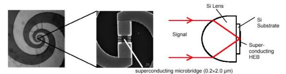
**Figure 3:** Superconducting NbN HEB: SEM picture of the planar logarithmic-spiral antenna with the superconducting microbridge in the center (left) and complete detector including the lens for coupling of the signal.
