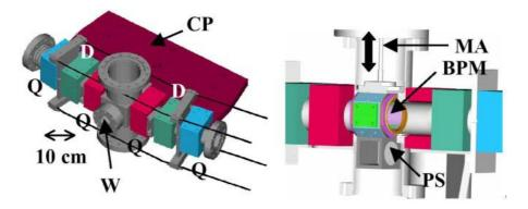
**Figure 2**: UMER  $20^{0}$  ring section (solid schematic on the left, and cut-out on the right). Q: Quadrupole, D: bending dipole, CP: cluster plate, W: viewing window, MA: mechanical actuator, BPM: beam-position monitor, PS: phosphor screen.
