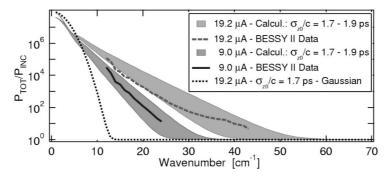
**Figure 3**: CSR gain as a function of the wavenumber. The BESSY II data for two different currents per bunch are compared with the shielded SR calculation and with the curve for a Gaussian distribution of the same length.
