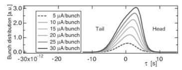
**Figure 2**: Calculated equilibrium distributions using the shielded SR wake. Case of the BESSY II in the configuration for CSR production.
