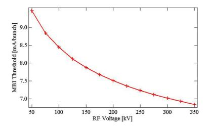
**Figure 1**: Single bunch average current threshold for the MBI calculated for DA $\Phi$ NE with  $E = 510 \text{ MeV}, \rho = 1.4 \text{ m}, \alpha_{C} = 0.02.$
