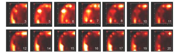
**Figure 14:** Series of spectral near-field images of the lesion region (upper left corner of the near-field image of Figure 12) between 3 and 20 cm-1 (between 0.5 and 3 mm wavelength). The corresponding wavenumber is indicated on top of each spectral frame.
