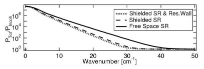
**Figure 4**: CSR gain vs. radiation wavenumber calculated using the shielded SR wake with (dotted line) and without (dashed line) the resistive wall wake. The solid line shows the gain calculated with the free space SR wake. Case of BESSY II with 9.0  $\mu$ A per bunch and 1.7 ps natural bunch length.
