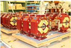
**Figure 4:** ATF2 quadrupole magnets fabricated by IHEP. Left – Magnets at IHEP under measurement; right – Magnets arrived at KEK.
