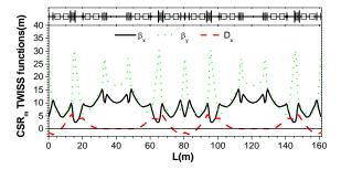
**Figure 2**:  $\beta$  and dispersion of CSRm
