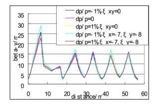
Figure 5: Vertical on- and off-axis beta function for one super-period
