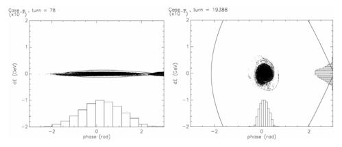
Figure 11: The longitudinal phase space at the initial and end of acceleration
