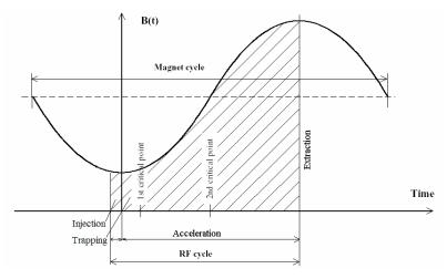
Figure 9: One cycle of magnetic field of RCS and its RF acceleration period
