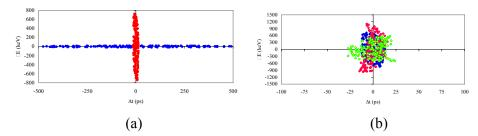
**Figure 1:** (a) the longitudinal emittance plots before and after the superbuncher in blue and red colours respectively; (b) the longitudinal emittance at the entrance, exit of the linac and on the target in blue, red and green colours respectively.
