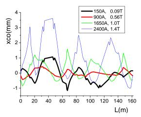
Figure 12: COD caused by dipole reproducibility.
