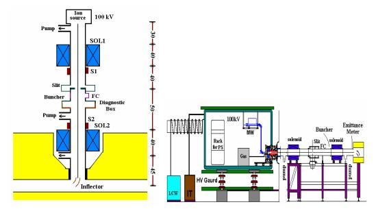
**Figure 10:** Scheme of injection and layout of the high voltage deck, source and Low Energy Beam Transport for preliminary study.
