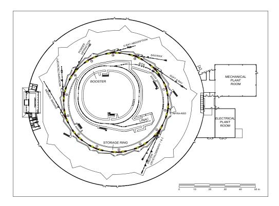
Figure 2: General layout of the Australian Synchrotron
