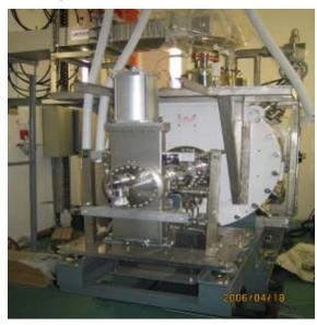
Figure 3: A RF cavity in test
