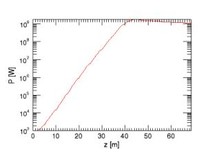
Figure 2: Power gain and saturation of PAL-XFEL.
