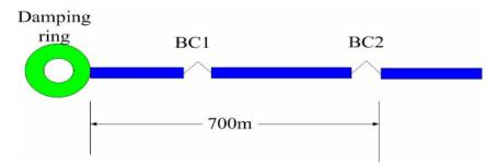
Figure 5: A schematic view of two-stage BC for ILC
