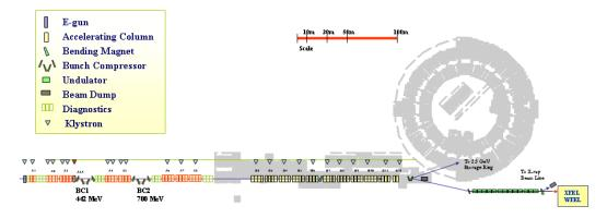
**Figure 1:** Layout of PAL-XFEL. The current linac building is shown in the figure. The beam transport dog-leg has approximately 0.5°, although it is exaggerated in the figure.
