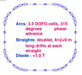
**Figure 3:** The geometry of RCS
