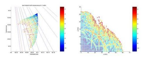
Figure 2: The FMA analysis of the working point of FODO4
