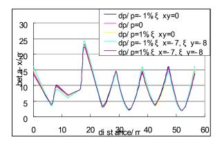
Figure 4: Horizontal on- and off-axis beta function for one super-period
