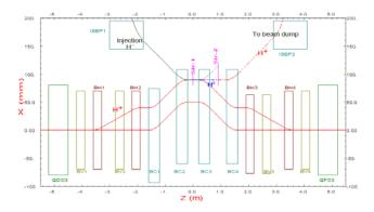
**Figure 7:** Injection scheme (BC1~BC4: closed-orbit bump magnets, BH1~BH4: horizontal painting bumpers, BV1~BV4: vertical painting bumpers, QDC3 & QFC3: quads, ISEP1&2: septa)
