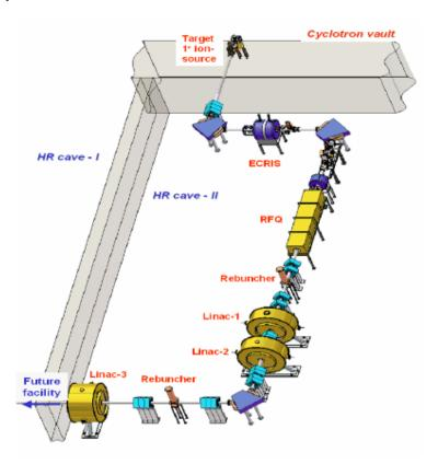
Figure 8: A schematic layout of the RIB facility to be built in Phase-1.
