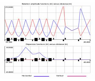
Figure 2: Twiss parameters for RCS lattice in one super-period
