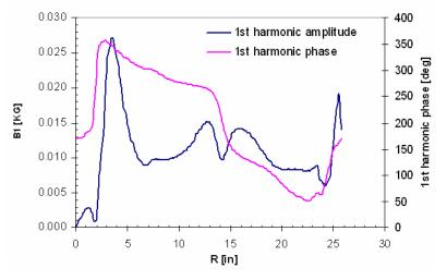
**Figure 7**: First harmonic field and amplitude ( $I_{\alpha} = I_{\beta} = 300 \text{ A}$ )
