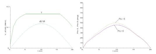
**Figure 10 :** The curves of RF voltage and energy gain during half RCS cycle(left), and the curves of RF phase (Phi-S) and bunch phase (Phi-B) (right)
