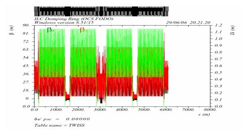
Figure 1: FODO lattice with 2 wiggler sections (FODO4)
