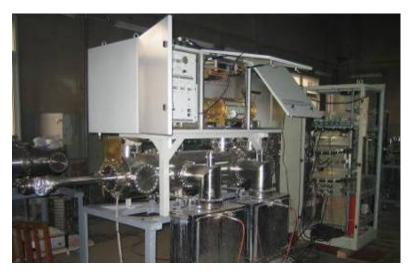
Figure 5: A kicker installed in the BEPCII tunnel
