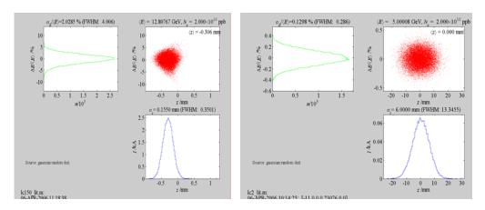
**Figure 6:** Bunch compressor design for ILC. Left – the bunch at the exit of ILC damping ring; right – the bunched beam at the exit of 2<sup>nd</sup> BC.
