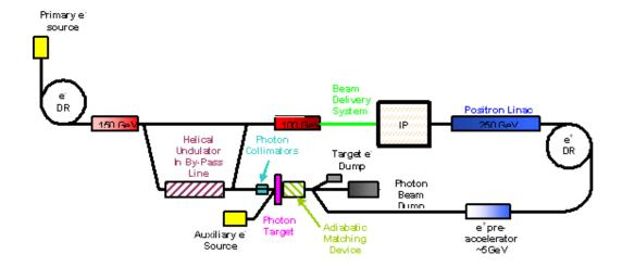
Figure 4: The helical undulator configuration for producing positrons for the ILC
