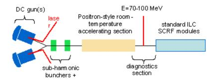
Figure 3: Configuration for the ILC Electron Source
