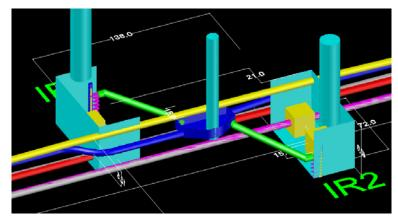
**Figure 6:** Baseline Configuration having two interaction regions with 138 m longitudinal separation
