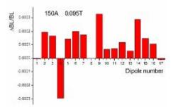
Figure 11: Reproducibility of CSRm dipole at 0.1T.
