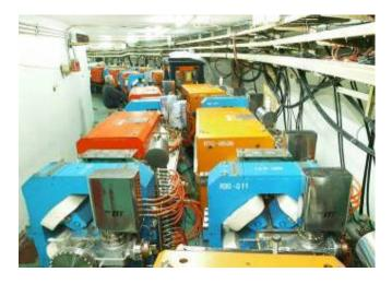
Figure 8: Installed accelerator units in the BEPCII tunnel
