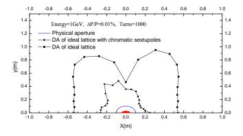
**Figure 4**: The DA of CSRm with error free.
