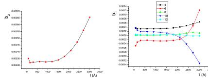
**Figure 6**: b<sub>2</sub>-coefficient versus the exciting current.
