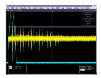
**Figure 1:** The injection kicker pulse (blue), and the first 30+ turns of electrons in the AS storage ring.
