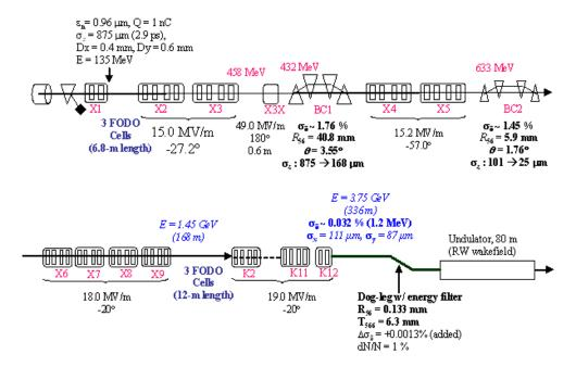
**Figure 3:** Layout of the PAL-XFEL injector and linac.
