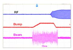
**Figure 20**: The synchronous signal between RF, bumping orbit and injection beam.
