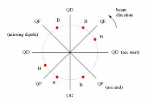
Figure 1: Dispersion suppression with a single missing dipole at each arc
