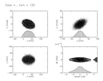
**Figure 8:** Beam distribution in phase spaces at the injection end (anti-correlated, Ip= 15mA, VRF=15kV)
