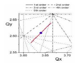
**Figure 3**: Tune distribution with  $\Delta P/P$  of  $\pm 0.6\%$
