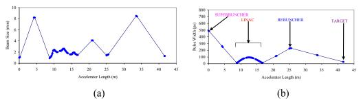
**Figure 2:** Through the length of the accelerator: (a) the beam size; and (b) the time envelop.
