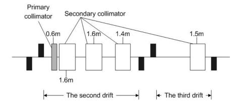
Figure 6: The layout of the transverse two-stage collimation system in the straight section
