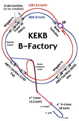
Figure 1: Schematic view of KEKB
