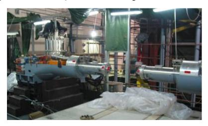
Figure 7: SCQ's and some warm magnets installed in IR
