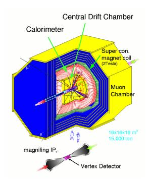
**Figure 7:** ILC Detectors will be  $4\pi$  detectors with precision tracking and calorimetry
