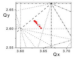
Figure 10: Tune-shift after the lattice modifying.
