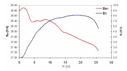
**Figure 6**: Average magnetic field and third harmonic field profile  $(I_{\alpha} = I_{\beta} = 300 \text{ A})$
