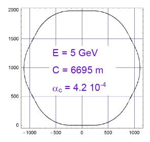
**Figure 5:** The Damping Ring has a six-fold symmetry with six straight sections. Four contain wigglers and RF cavities; one has injection and extraction systems, while the final one has the abortion line. The arcs each have 18 TME cells and dispersion suppression.
