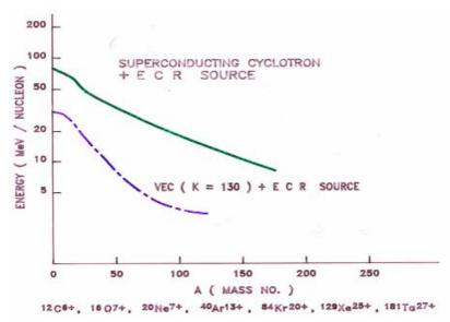
**Figure 4:** Energy/nucleon vs mass number for heavy ion beams at the VEC Centre.
