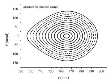
Figure 3: Dynamic aperture in the horizontal direction for the POP-FFAG.
