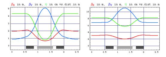
Figure 4: Lattice Functions along the length of a period (Project D).
