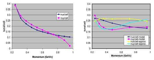
**Figure 4:** Dependence of cell tunes on momentum in LNS-FFAGs: (left) conventional design for rapid, or muon, acceleration; (right) tune-stabilized for medical therapy [36]. In the legend, approx refers to an analytic solution, model to one obtained using MAD.
