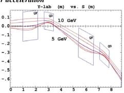
Figure 6: Muon FFAG cell and closed orbits
