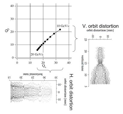
Figure 3: Tune excursion of 10 to 20 GeV/c muon ring and orbit distortion when alignment errors of 0.1 mm (rms) are included.
