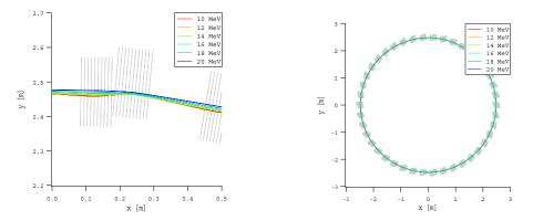
Figure 2: Closed orbits in EMMA for several fixed energies.
