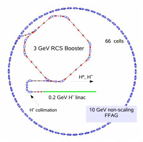
**Figure 5:** Schematic layout drawing of the linac, booster and NFFAG of the proton driver. It is recommended that a low energy electron model of the ring be constructed and
