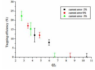
**Figure 4:** Trapping efficiency measured at POP-FFAG (crossing  $3Q_x=7$ ). The horizontal axis  $\alpha_1$  is proportional to  $(\epsilon/\Delta e)^{2/3}$ , where  $\epsilon$  is the crossing speed and  $\Delta e$  is the resonance width. Details are shown in [9].
