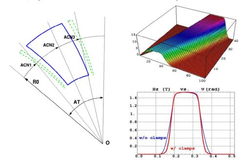
**Figure 2:** Left: geometry of a spiral sector dipole and typical ingredients (angles, radius, etc.) to define the optical element and positioning of its EFBs, including possible field clamps (dotted lines). Right, top: 3-D representation of the field as delivered by the "FFAG-SPI" procedure; bottom: field fall-off, together with the effect of the clamp modelling.
