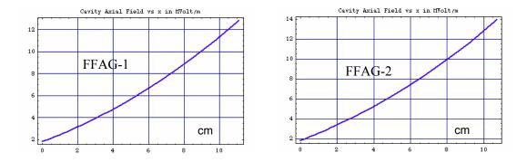
Figure 5: Total Surface Axial Field for each rf Cavity.
