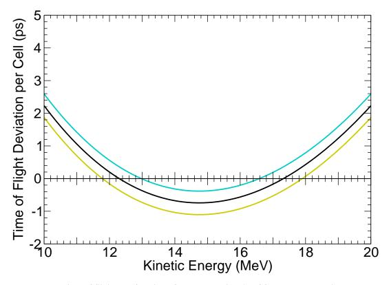
Figure 7: Time of flight as a function of energy, varying the rf frequency. Zero time means that the particle following the energy-dependent closed orbit is synchronized with the rf.
