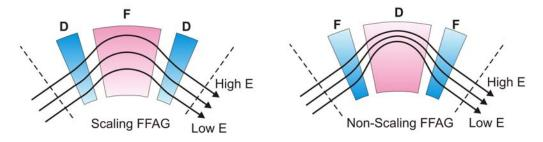
**Figure 2:** Scaling and non-scaling FFAG magnetic fields and orbit patterns. Positive-bending fields are shown in pink, negative in blue, with the colour density indicating the field strength. Note that FDF scaling and DFD non-scaling lattices are also possible.
