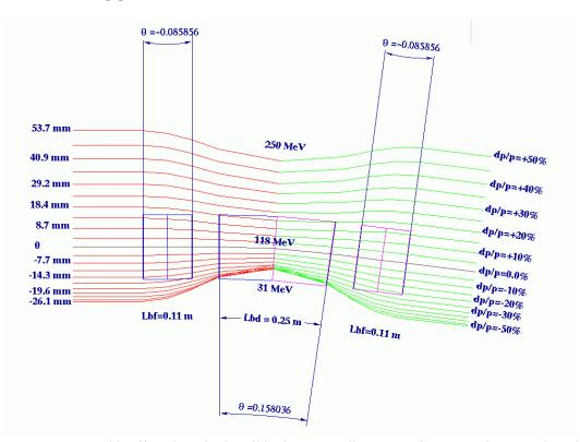
**Figure 2:** Orbit offsets in a single cell in the non-scaling FFAG for proton therapy. The cell length is 0.9 m; there are 48 cells with circumference 43.2 m. Drift lengths between the magnets are 6 cm long, while drifts for the extraction/injection and cavity length are 31 cm. Orbits are obtained from the Polymorphic Tracking Code (PTC) [4].
