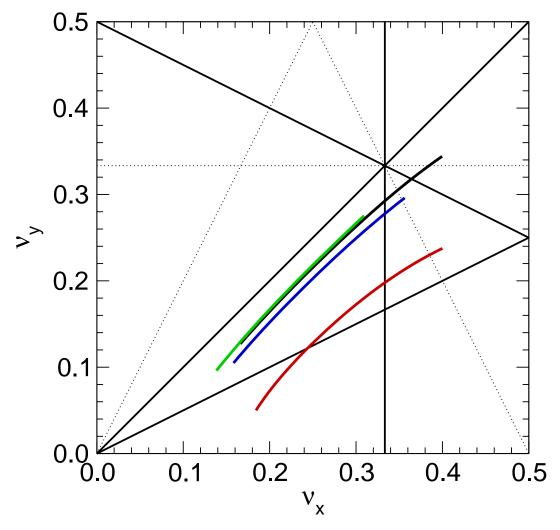
**Figure 1:** Single-cell tune as a function of energy for four different EMMA lattice configurations. Also shown are resonance lines to third order. Dotted lines are third-order resonances that are driven by skew sextupoles. Higher tunes are lower energy.
