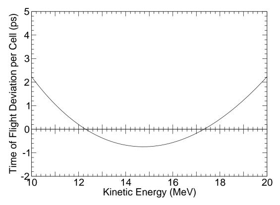
**Figure 2:** Time of flight as a function of energy in a single linear non-scaling FFAG cell. Zero time of flight deviation means that the time of flight is an integer number of rf wavelengths.
