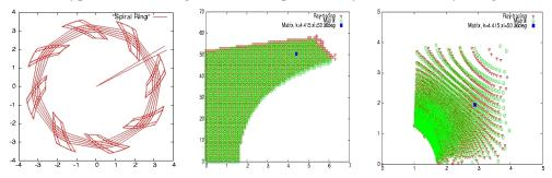
**Figure 4:** Left: spiral lattice ring, diameter ~7 m, maximum field 1.5 T on high energy orbit, packing factor 0.38. Middle: a scan of the stability domain in the k (field index, horizontal axis) and q (spiral angle, vertical axis) variables. Left: the corresponding stability region in the tune diagram.
