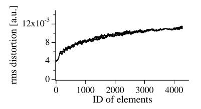
Figure 4: RMS orbit distortion out of 501 tracking results.
