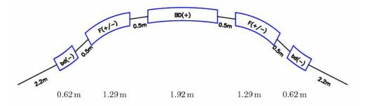
Figure 3: A single lattice cell of the 50 Hz, 4 MW, 10 GeV, NFFAG proton driver ring.
