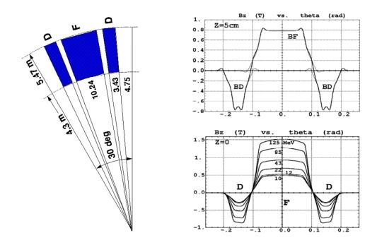
**Figure 1:** Left: geometry of the KEK 150 MeV radial scaling DFD FFAG triplet. Right, top: magnetic field across the triplet on an arc of a circle, at non-zero z, using the "FFAG" procedure, as obtained by superposition (thick line) of the independent contributions (thin lines). Right, bottom: field on closed orbits in the 12-cell ring, from 10 to 125 MeV.
