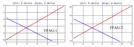
Figure 6: Field Profiles (kG) in the two FFAG Rings vs. Radial location x (cm) (Project D).
