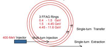
Figure 2: Schematic layout of a proposed FFAG for a Neutrino Factory.
