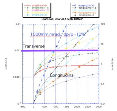
Figure 8: Transverse and longitudinal emittance growth in ERIT.
