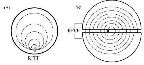
**Figure 1:** Sketch of a Microtron (A) where all the trajectories with increasing radii go through the same location of the accelerating rf cavity, and of a Cyclotron (B) where the trajectories spiral toward to larger radii and traverse a region where rf accelerating field is applied.
