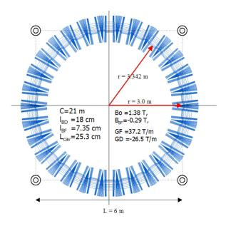
**Figure 7:** Non-scaling FFAG ring with triplet magnet cells as a possibility for the Oxford University proton medical accelerator. The protons are accelerated from the kinetic energy of 11.6 to 100 MeV.
