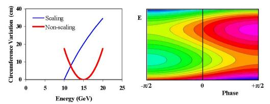
Figure 3: Linear non-scaling FFAGs. (Left): Circumference variation with energy. (Right): Acceleration path (yellow) in longitudinal phase space.
