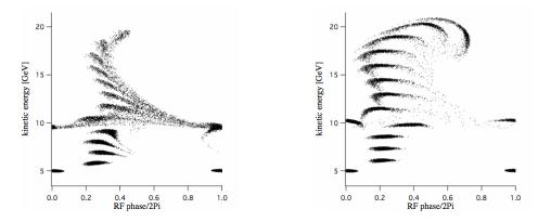
**Figure 5:** Longitudinal emittance evolution in a cascade of two FFAG with transverse emittance of 30  $\pi$  mm rad. First FFAG accelerated from 5 to 10 GeV and the second does from 10 to 20 GeV. Left figure uses nominal rf voltage and no higher harmonic rf. Right figure uses second harmonic rf with 10% increase in fundamental rf voltage.
