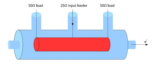
Figure 2: Broadband, centre-fed (or travelling wave), drift tube rf system.
