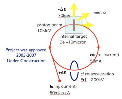
Figure 7: Schematic diagram of ERIT.
