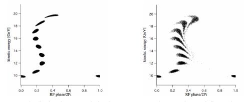
Figure 5: Longitudinal emittance evolution in a 10 to 20 GeV/c muon ring. Left figure shows a beam with zero transverse emittance and right figure shows a beam with  $30 \pi$  mm rad.
