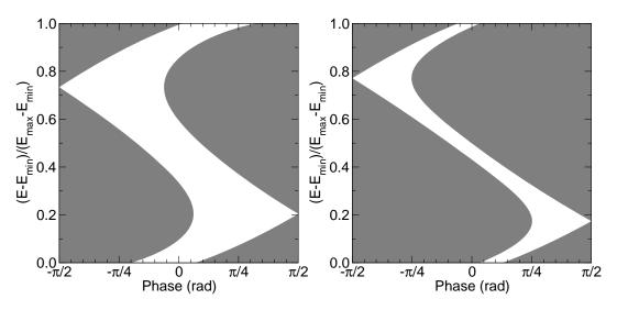
Figure 8: Longitudinal phase space when the time of flight is synchronized with the rf at different energies. The white region is the region of phase space through which particles are transmitted.
