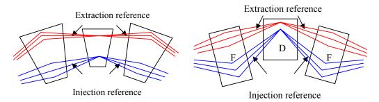
**Figure 2:** 1½ cells of a non-scaling, linear-field FFAG which is tune-stabilized for medical therapy (left) compared with 1½ cells of a doublet-based non-scaling FFAG (right) for muon acceleration.
