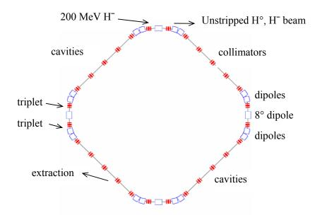
Figure 1: Schematic layout drawing of the 50 Hz, 1.2 MW, 3 GeV, booster synchrotron.
