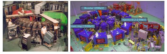
**Figure 1:** Scaling FFAGs. (Left): 50-MeV electron model at MURA in 1961. (Right): The three proton rings for ADSR studies at Kyoto University Research Reactor Institute in 2006.
