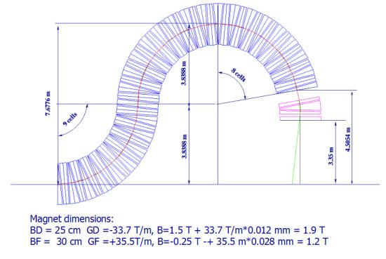
**Figure 8:** Proton gantry made of non-scaling FFAG cells with a magnetic field sufficiently small that permanent magnets can be used. Superconducting magnets made without any iron could be used to reduce the size (perhaps by as much as a factor of two).
