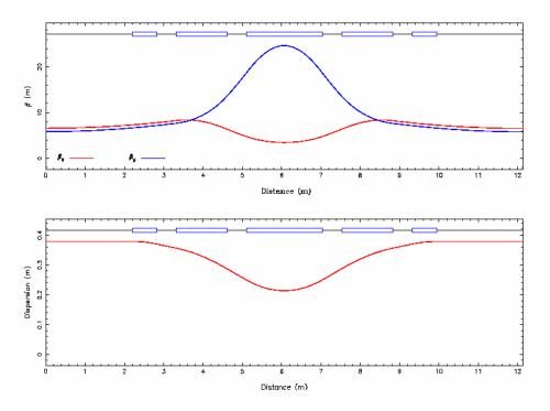
Figure 4: Small amplitude betatron and dispersion functions for the NFFAG 10 GeV orbit
