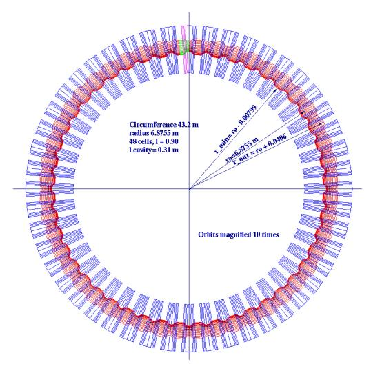
and minimum orbit offsets at the magnet aperture, the gradient and the variation of the magnetic field in the transverse direction.
