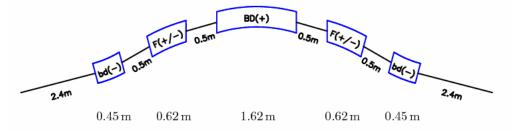
Figure 1: Schematic Layout of the 10.2 m Lattice Cell for the 20 GeV Orbit.
