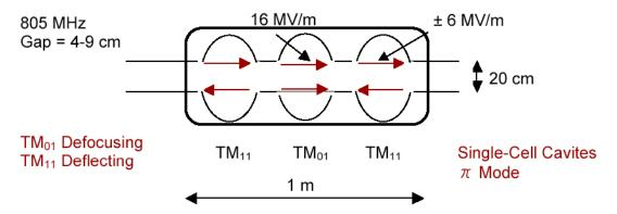
Figure 6: Combination of 3 cavities to reproduce behavior of required axial field profile.
