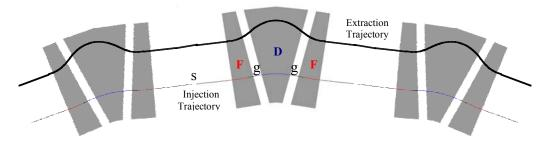
Figure 3: The FDF-Triplet Period of a FFAG Ring.
