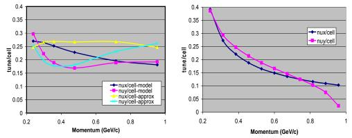
**Figure 1**: Dependence of cell tune on momentum in a non-scaling, linear-field FFAG which is tune-stabilized for medical therapy. In the legend, 'approx' means the solution obtained from solving a set of approximated optical equations and 'model' means the tune as modeled in MAD using solutions found for the CF magnetic fields. Dependence of cell tune on momentum in a linear-field FFAG designed for rapid, or muon, acceleration is shown on the left.
