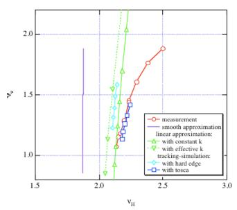
**Figure 2:** Tune diagram of the POP-FFAG for different operating conditions. The red open circles and the blue squares show the measured values and the beam tracking results with the TOSCA-OPERA field simulation, respectively.
