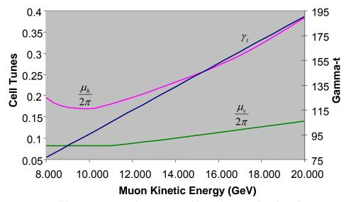
Figure 2: Cell betatron tunes and gamma-transition values as a function of muon energy.
