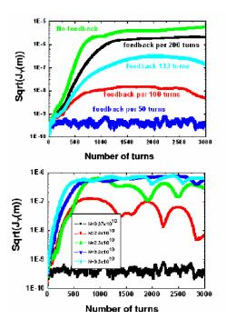
Figure 3: Vertical amplitudes with different number of feedback (top) and different currents (bottom).
