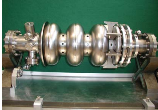
Figure 5: Photograph of the 3-1/2-cell SRF gun cavity.
