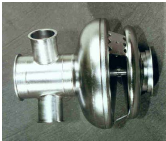
Figure 2: Half-cell cavity of the first operating SRF gun at Rossendorf [27].
