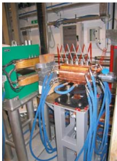
Figure 12: RF deflector cavity installed in the SPARC machine.
