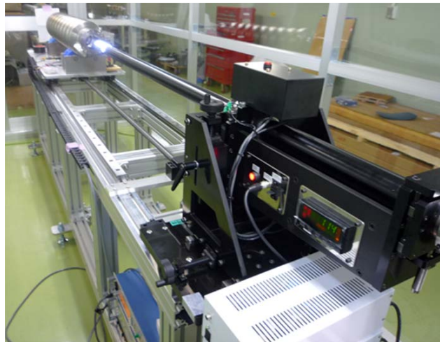
Figure 7: The upgraded inspection camera system for cavity inner surface observation.
