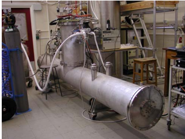
Figure 3: The 4m long cryomodule under commissioning at RAL.
