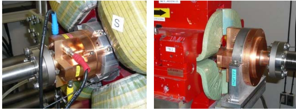
Figure 15: C-band cavity BPM in the ATF2 quadrupole (left) and S-band cavity BPM in the final doublet quadrupole (right).
