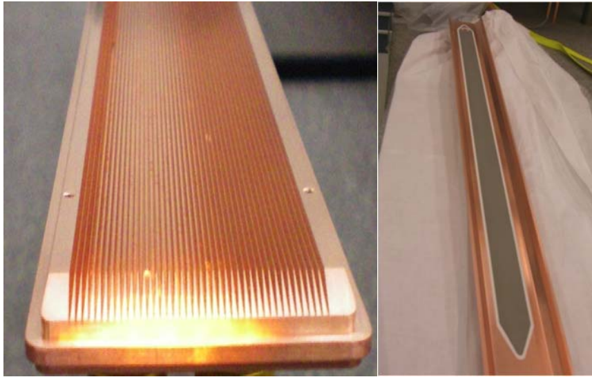
Figure 5: Left: a grooved Cu insert with 21.8^\circ triangular grooves having 1mm pitch for testing in a CESRTA wiggler. Right: a thin clearing electrode applied with a thermal spray method to the bottom half of another CESRTA experimental wiggler chamber.
