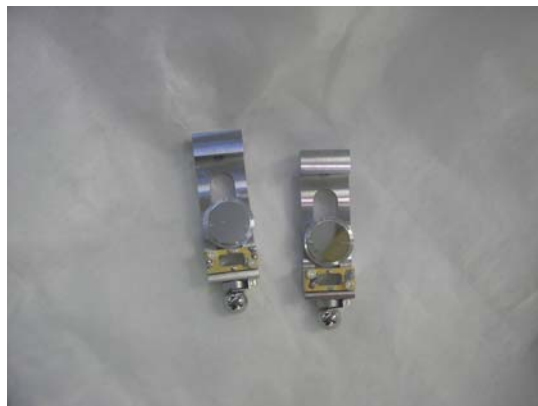
Figure 5: Target holders and wire cards with the targets.
