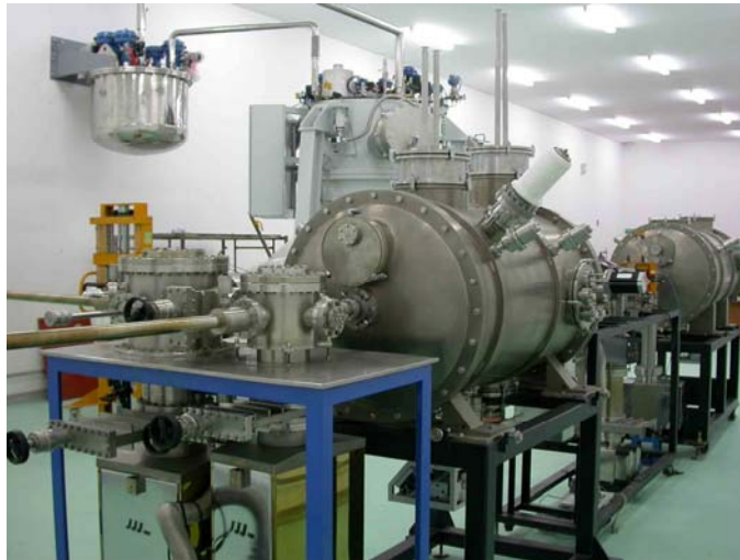
Figure 4: Cryomodule of DC-SF injector and the main accelerator
