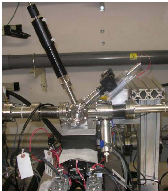
Figure 6: OTR with the calibration system installed at ATF2.
