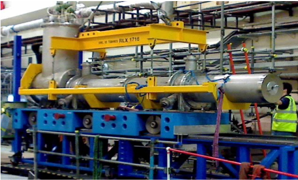
Figure 6: Photo of Decay Solenoid prior to its installation into the ISIS-vault shielding wall.
