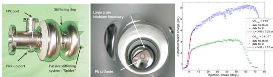
Figure 6: (left) 1/2 -cell SRF photoinjector designed by DESY and produced at Jefferson Lab. with (middle) Pb-coated backplane acting as a SC cathode (coating at NCBJ, Swierk). (right) Measured extracted bunch charge versus emission phase for two different regions of the photocathode, yielding bunch lengths of order 3 ps.
