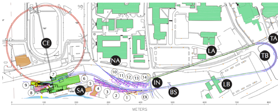
Figure 1: Cornell ERL layout with section labels in black disks. Circled numbers indicate undulators and their corresponding x-ray beamlines. The existing Wilson Lab will house undulators 7-9, while a new x-ray science building will house the remaining eleven undulators, as well as the injector and an extracted beamline (EX). The Linac sections LA and LB and turnaround arc TA and TB will occupy a single tunnel.
