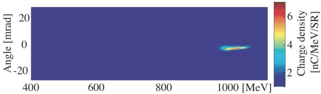
Figure 1: Single-shot electron beam spectrum from a 310-micron diameter H-discharge capillary with on-axis density 4 \times 10^{18} \text{ cm}^{-3} and a 1.5 J, 46 fs laser. The H-discharge capillary forms a plasma channel for guiding the laser. The 1012 MeV electron beam contained 30 pC of charge, with 2.9% (rms) energy spread and 1.7 mrad (rms) divergence.
