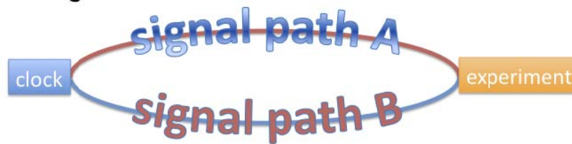
Figure 4. Two timing signal paths with different delays to the experiment.
