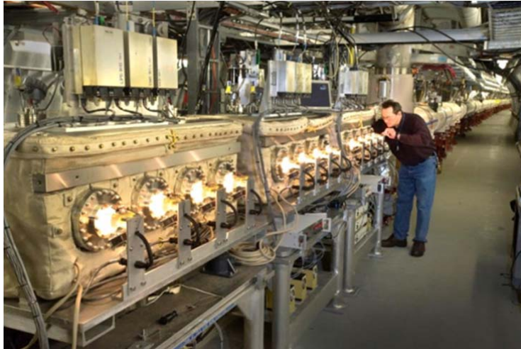
Figure 6: The three vacuum tanks of the new longitudinal kickers for the blue ring. Spot lights shine through glass windows to keep the cavities at 50 C.
