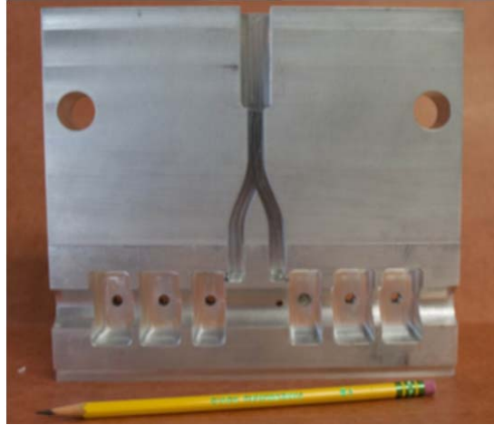
Figure 1: Prototype of 6 GHz 6-cell kicker cavity. One half of the cavity is shown. Waveguide splits to feed the two 3-cells in phase.
