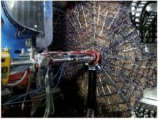
**Figure 3:** Additional carbon fiber composite legs (central black poles) superimposed to the original low-β support structure.
