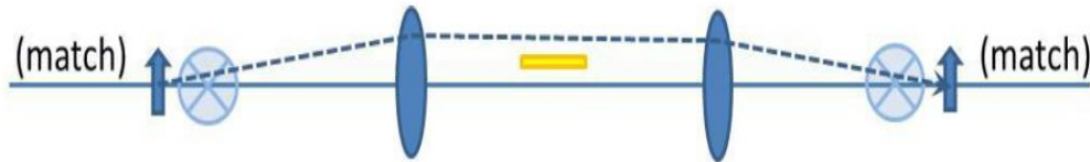
Figure 8: Orbit configuration and beam handling sequence for recirculated beam. Beam motion is from left to right.
