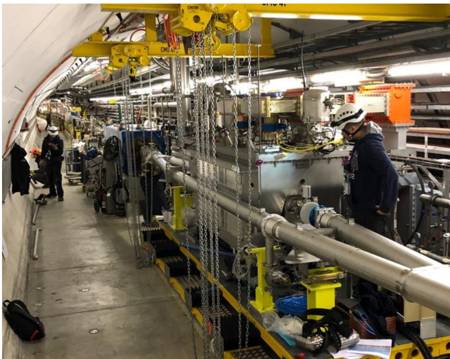
Figure 34: The LHC prototype twin DQWCC cryomodule installed in the SPS tunnel for beam tests.
