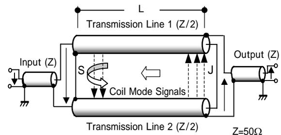
Fig.1. The basis of the structure of the TLBT.
