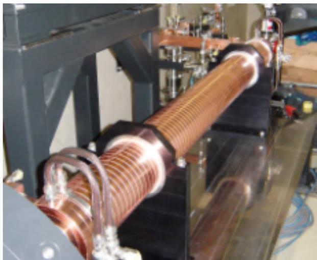
Fig.1: Photograph of the C-band accelerating structure for the SCSS project.
