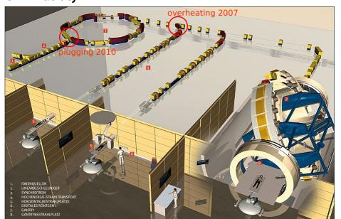
The Heidelberg Ion Beam Therapy Centre with 1. ion sources, 2. linear accelerator, 3. synchrotron, 4. high energy beam transport line, 5. horizontal treatment rooms, 6. digital x-ray imaging, 7. gantry, 8. gantry treatment room.
