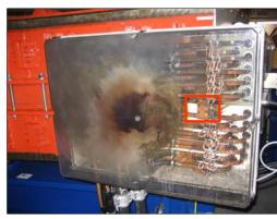
Connection box of first 45° dipole into the first horizontal treatment room after overheating.
