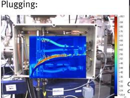
Thermal image of water circuits with persisting plugging (scale max. 89.1 °C)
