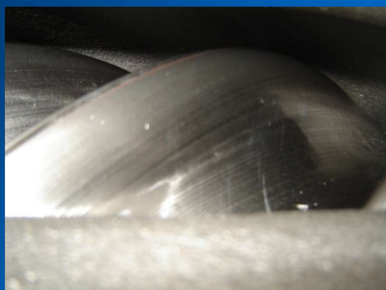
View of the screw compressor from the inside
