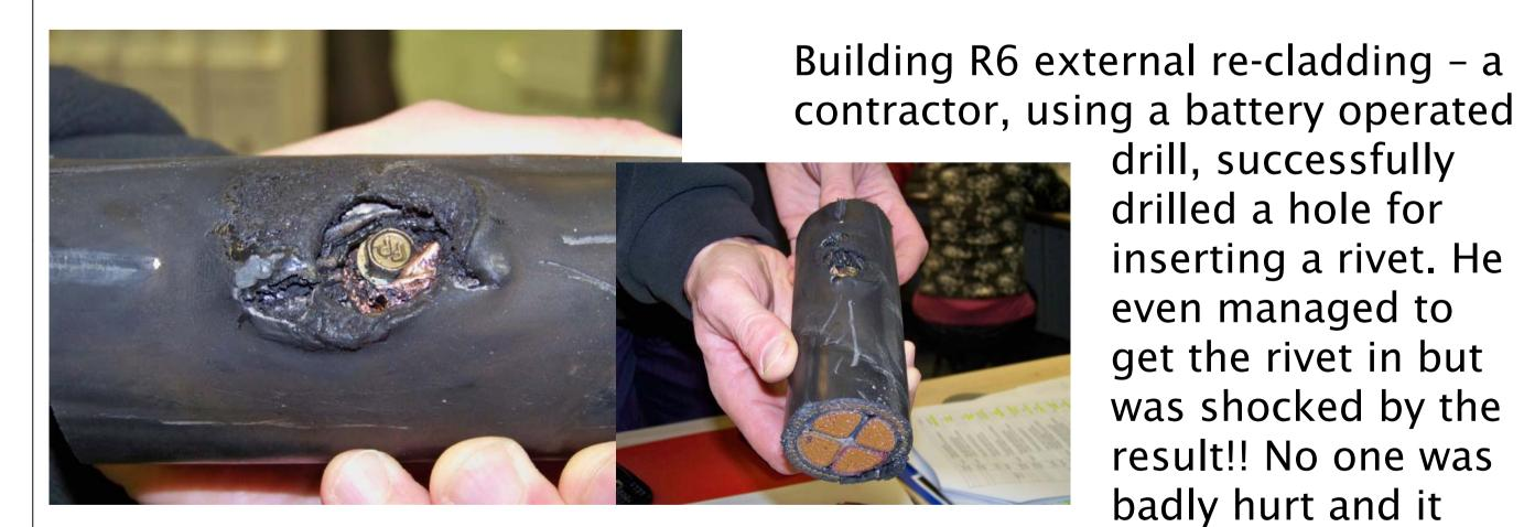
drill, successfully drilled a hole for inserting a rivet. He even managed to get the rivet in but was shocked by the result!! No one was badly hurt and it took 4 hours to
