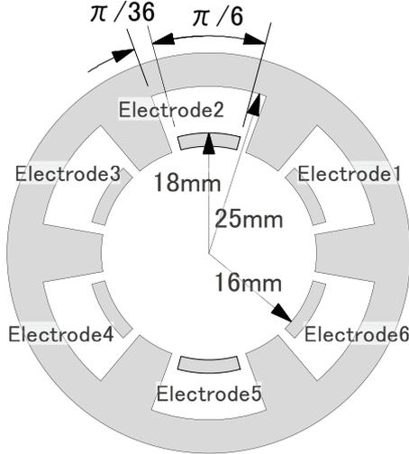
Figure 2: Dimension of BPM with circular cross-section.
