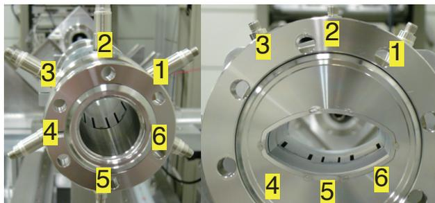
Figure 1: Six-electrode BPMs with circular and quasi-elliptical cross-sections for SPring-8 linear accelerator. Numbers represent electrode number  $d$ .
