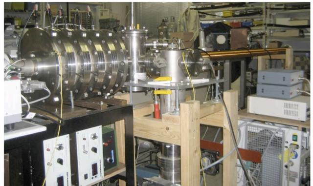
Figure 1: Experimental apparatus for bunch compression by induction modulator in Tokyo Institute of Technology.
