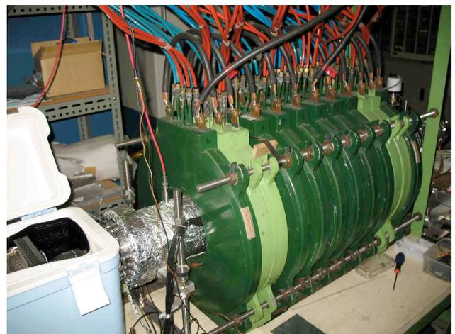
Figure 4: Experimental apparatus by Malmberg-Penning trap for bunch compression in Kanazawa University.
