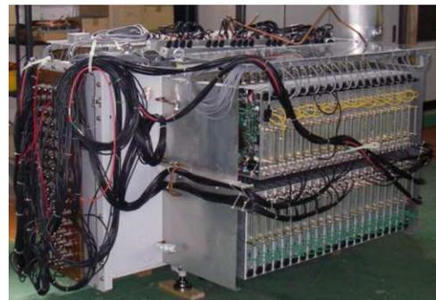
Figure 2: Induction accelerator modules.
