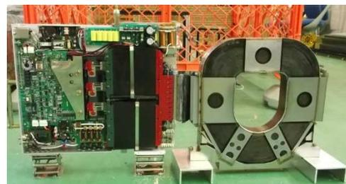
Figure 3: IGBT and an induction core.
