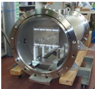
Figure 6a: 20 kV Electrostatic Injection Kicker
