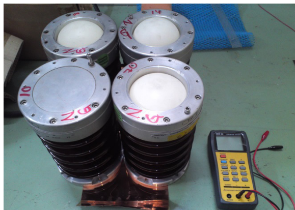
Figure 6: Photograph of damaged capacitances used in a PFN of a klystron modulator and an LCR meter used to check the capacitance. The explosion proof valves of three capacitances are already opened.
